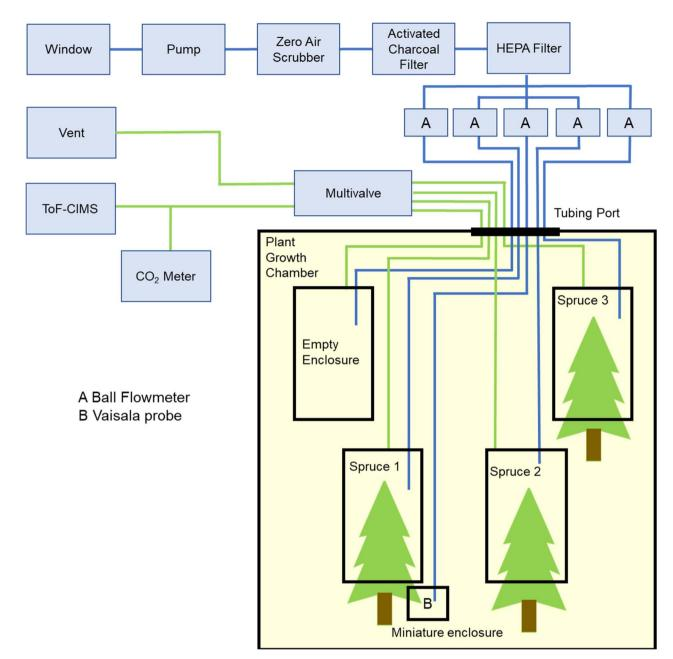
Fig. 1 Schematic of emissions sampling set-up.
