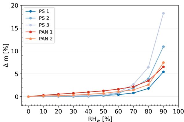
Fig. 4 Water vapour uptake isotherms shown as relative sample mass change as a function of  $RH_w$  measured by DVS at  $T = 298.5$  K. Data points represent water uptake at quasi-equilibrated relative humidity conditions. The curves are linear interpolations between the points. Each curve represents once one adsorption and one desorption cycle taking a total of 5 days per sample.
