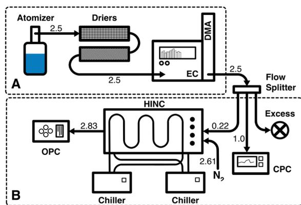
Fig. 1 Schematic of the experimental setup. (A) Aerosolization of the sample and size selection of the NP. (B) Ice nucleation experiment. The numbers indicate the flow rates in L min<sup>-1</sup>.
