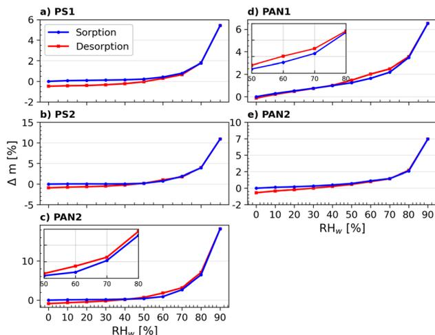
Fig. 5 Water vapor uptake and loss isotherms shown as relative sample mass change as a function of  $RH_w$  measured by DVS at  $T = 298.5$  K. Data points represent water uptake at quasi-equilibrated relative humidity conditions. The curves are linear interpolations between the points. Note different y-axis range on panels.
