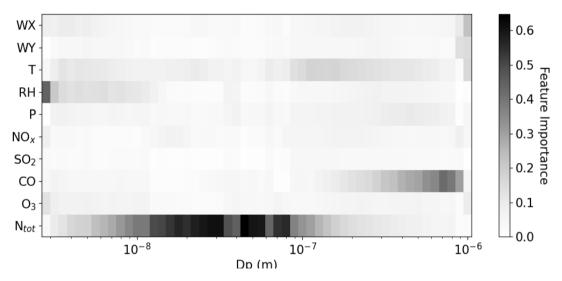
Random forest feature importance (WX: north component of horizontal wind speed and WY: east component of horizontal wind speed).
