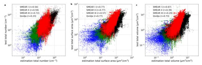
Fig. 3 Comparison of estimated versus test data for variables derived from the particle number size distribution across multiple sites. (a) Total number concentration (cm $^{-3}$ ), (b) total surface area ( $\mu$ m $^2$  cm $^{-3}$ ), and (c) total volume ( $\mu$ m $^3$  cm $^{-3}$ ). Each point on the plot represents a paired comparison between the model's estimation and the corresponding measured value. The color of the points indicates the station where the data was collected
