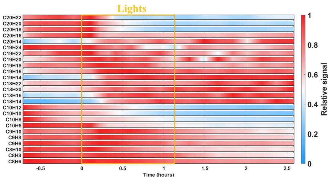
Fig. 3 Evolution of the relative signal of particle-phase species during the low- $NO_x$  experiment, with compounds grouped by carbon and hydrogen numbers. Red indicates that the species are close to their maximum relative intensity, while blue signals a low relative intensity. UV lights are indicated by the yellow box.
