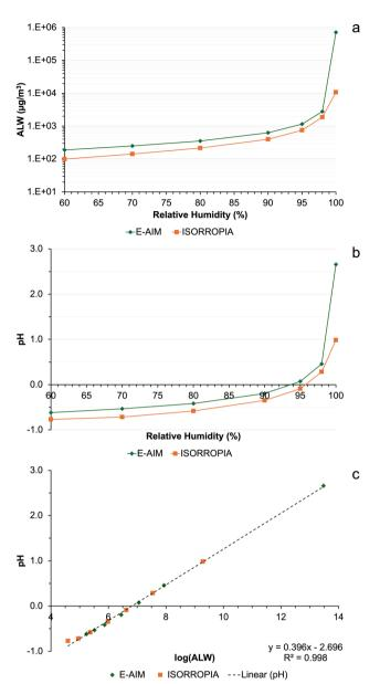
Fig. 2 Comparison of the outputs between E-AIM and ISORROPIA using the chemical composition of sample S1-0807-PM<sub>0.5-0.25</sub> (summit 1,  $0.5-0.25 \mu m$  size fraction) as the input and varying relative humidity, between 60% and 100%: (a) aerosol liquid water (ALW) content, (b) pH, and (c) correlation between ALW and pH.
