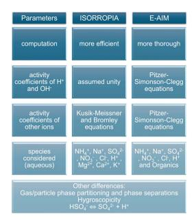
Fig. 3 Infographic summarising the main known differences between the thermodynamic calculations of aerosol liquid water content and pH by the ISORROPIA and E-AIM models.
