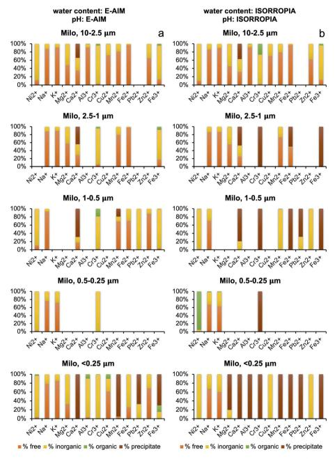
Fig. 6 Comparison of metal speciation estimated with Visual MINTEQ and based on samples collected in Milo, 10 km downwind of the plume, using (a) water content and pH calculated with E-AIM, and (b) water content and pH calculated with ISORROPIA.
