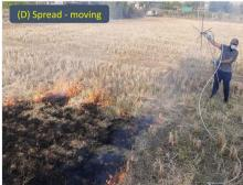
Fig. 1 Photographs of crop residue burning emission measurements showing different configurations of the multi-arm inlet: (A) piled residue with vertical advection of plume, (B) piled residue with horizontal advection of wind, (C) spread residue with a static inlet with vertical configuration, and (D) spread residue with a moving multi-arm inlet.
