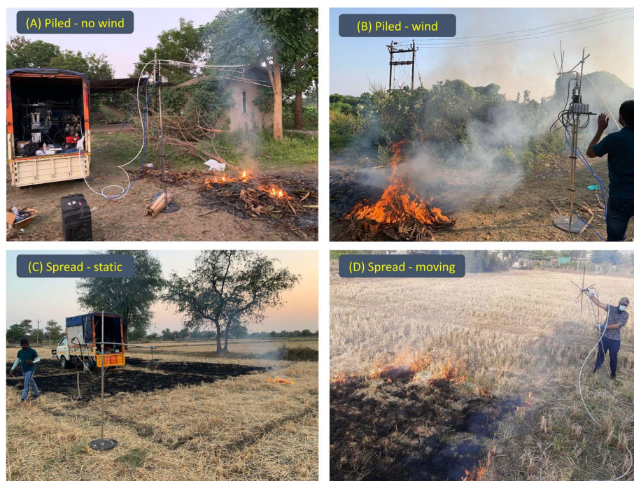
Fig. 1 Photographs of crop residue burning emission measurements showing different configurations of the multi-arm inlet: (A) piled residue with vertical advection of plume, (B) piled residue with horizontal advection of wind, (C) spread residue with a static inlet with vertical configuration, and (D) spread residue with a moving multi-arm inlet.
