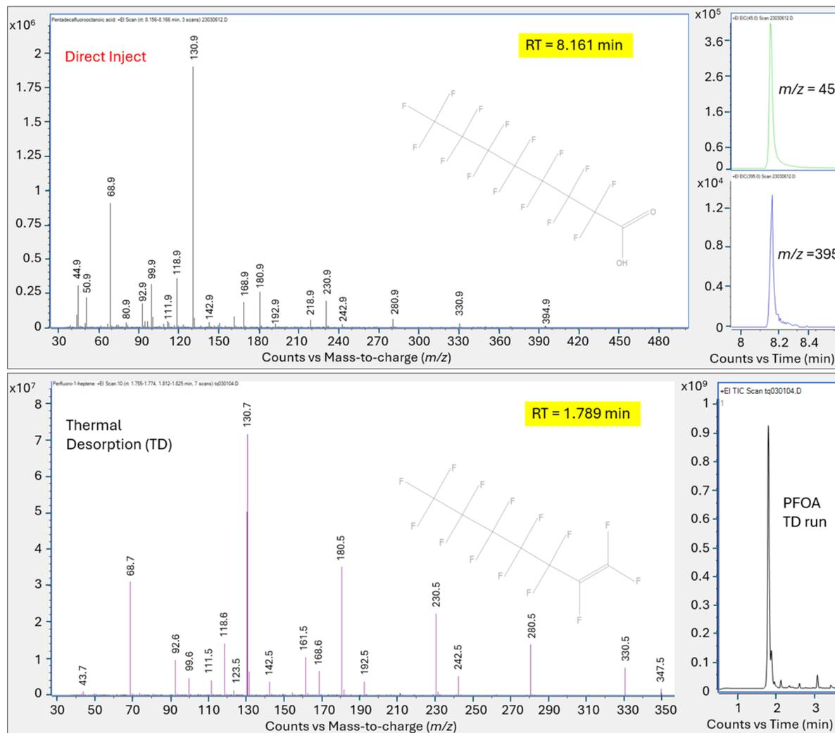
Fig. 4 Mass spectra for primary peak measured from PFOA injection using direct injection and TD on HP-5MS column; X axis is mass to charge ratio, y axis is counts; Upper panel is direct injection method, bottom panel is thermal desorption, right inset shows chromatogram.
