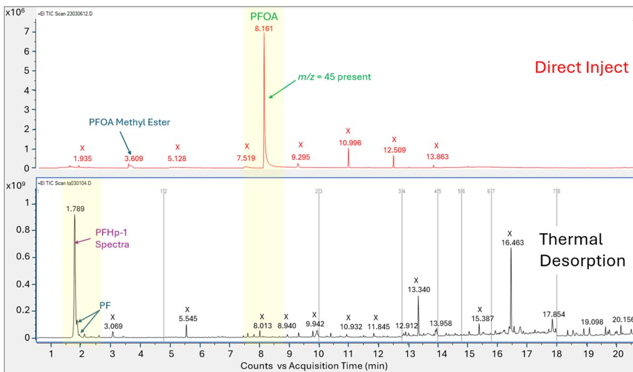
Fig. 3 Total ion chromatograms for PFOA analysis on HP-5MS column with direct injection (top panel) vs. thermal desorption (bottom panel); area counts on Y axis, and retention time in minutes on the x axis, labels on figure are X = non-perfluorinated compound; PF = perfluorinated compound, identified structures labeled.
