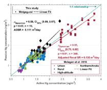
Fig. 3 Spearman correlation of active in situ measurement against MerPAS® OSR and AOSR in this study and PAS-derived Hg concentrations using Mclagan et al. 2018 recalibrated SR and adjusted SR. The inferential statistics, an estimate of effect size and uncertainty, and pairwise comparisons are also shown. The dotted lines represent the trend line for each dataset. The dashed dark teal line is the 1:1 relationship
