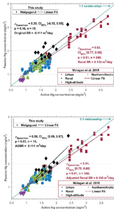
Fig. 3 Spearman correlation of active *in situ* measurement against MerPAS® OSR and AOSR in this study and PAS-derived Hg concentrations using McLagan *et al.* 2018 recalibrated SR and adjusted SR. The inferential statistics, an estimate of effect size and uncertainty, and pairwise comparisons are also shown. The dotted lines represent the trend line for each dataset. The dashed dark teal line is the 1:1 relationship.
