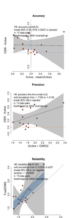
Fig. 4 Similarity of accuracy (top panel), precision (middle panel), and reliability (bottom panel) for active in situ vs. MerPAS® OSR obtained with  $5 \times 10^3$  bootstrap iterations.
