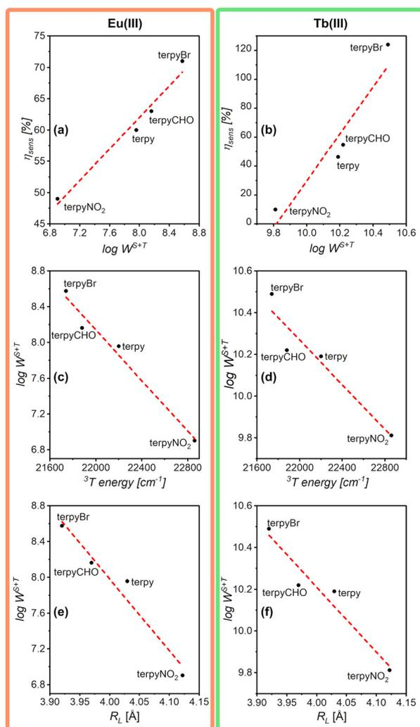
**Fig. 6** Correlation between energy transfer rates and different parameters. Correlations related to the Eu(terpyR) complexes, between the logarithm of total forward transfer rates and sensitization efficiency (a), ligand triplet energy (b), donor–acceptor distance (c). Correlations related to the Tb(terpyR) complexes, between the logarithm of total forward transfer rates and sensitization efficiency (d), ligand triplet energy (e), and donor–acceptor distance (f).
