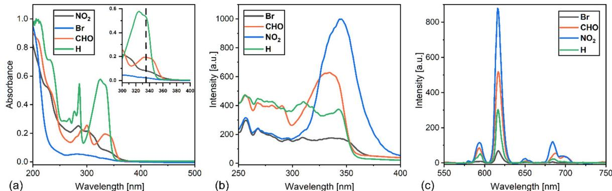
Fig. 3 Absorption (a), excitation (b), and emission (c) spectra of Eu-terpyR complexes [R = H (green), NO<sub>2</sub> (black), Br (blue), and CHO (red)] in acetonitrile at 298 K.  $\lambda_{\text{exc}} = 335$  nm,  $\lambda_{\text{em}} = 617$  nm, slit widths excitation = emission = 5 nm; scan rate = 250 nm min<sup>-1</sup>; gain = 650 V; [complexes] = 0.10 mM.
