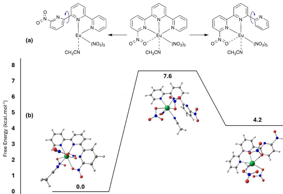
**Fig. 8** (a) Three structures considered for the Eu(terpyNO<sub>2</sub>) complex representing isomerization via decomplexation. (b) The free energy surface for the de-coordination of the pyridine nitrogen in the Eu(terpyNO<sub>2</sub>)(NO<sub>3</sub>)<sub>3</sub> complex. The structure on the left, right and middle are the geometries of the bound complex, unbound complex and the transition state structure respectively.
