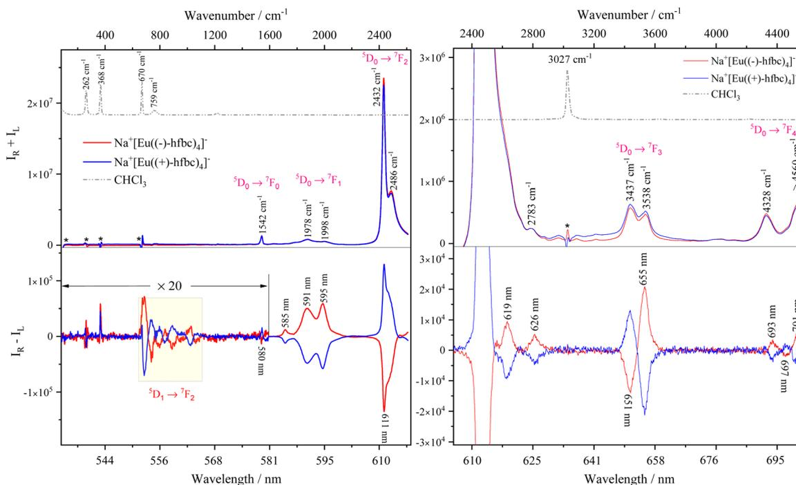
**Fig. 6** Raman/luminescence ( $I_R + I_L$ ) and ROA/CPL ( $I_R - I_L$ ) spectra of  $Na^+[Eu(\pm)-hfbc)_4]^-$  enantiomer complexes (3 mM) in chloroform in the range of  $80$ – $2630$   $cm^{-1}$  (left) and  $2280$ – $4580$   $cm^{-1}$  (right). Minor artifacts (marked by asterisks [\*]) are due to subtracting the chloroform signal.
