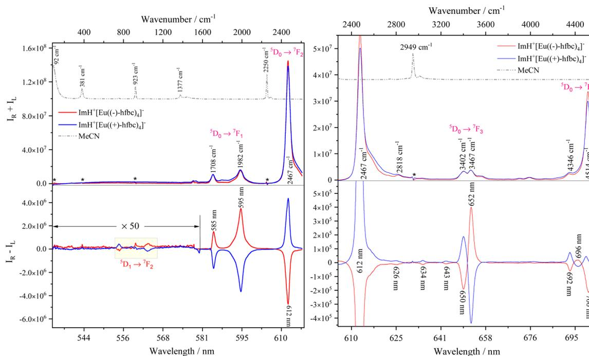
Fig. 5 Raman/luminescence ( $I_R + I_L$ ) and ROA/CPL ( $I_R - I_L$ ) spectra of  $\text{ImH}^+[\text{Eu}(\pm\text{-hfbc})_4]^-$  enantiomer complexes (1 mM) in acetonitrile in the range of 80–2630  $\text{cm}^{-1}$  (left) and 2280–4580  $\text{cm}^{-1}$  (right). Minor artifacts (marked by asterisks [\*]) are due to subtracting the acetonitrile signal.
