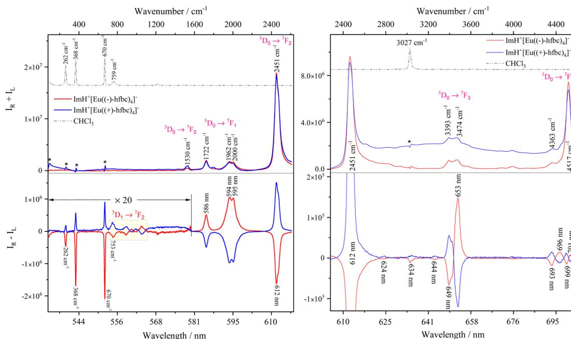
Fig. 4 Raman/luminescence ( $I_R + I_L$ ) and ROA/CPL ( $I_R - I_L$ ) spectra of  $\text{ImH}^+[\text{Eu}(\pm\text{-hfbc})_4]^-$  enantiomer complexes (3 mM) in chloroform in the range of 80–2630  $\text{cm}^{-1}$  (left) and 2280–4580  $\text{cm}^{-1}$  (right). Minor artifacts (marked by asterisks [\*]) are due to subtracting the chloroform signal.
