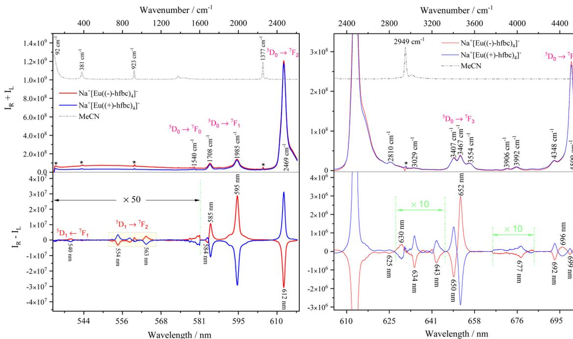
**Fig. 7** Raman/luminescence ( $I_R + I_L$ ) and ROA/CPL ( $I_R - I_L$ ) spectra of  $\text{Na}^+[\text{Eu}(\pm)\text{-hfbc}_4]^-$  enantiomer complexes (1 mM) in acetonitrile in the range of 80–2630  $\text{cm}^{-1}$  (left) and 2280–4580  $\text{cm}^{-1}$  (right). Minor artifacts (marked by asterisks [\*]) are due to subtracting the acetonitrile signal.
