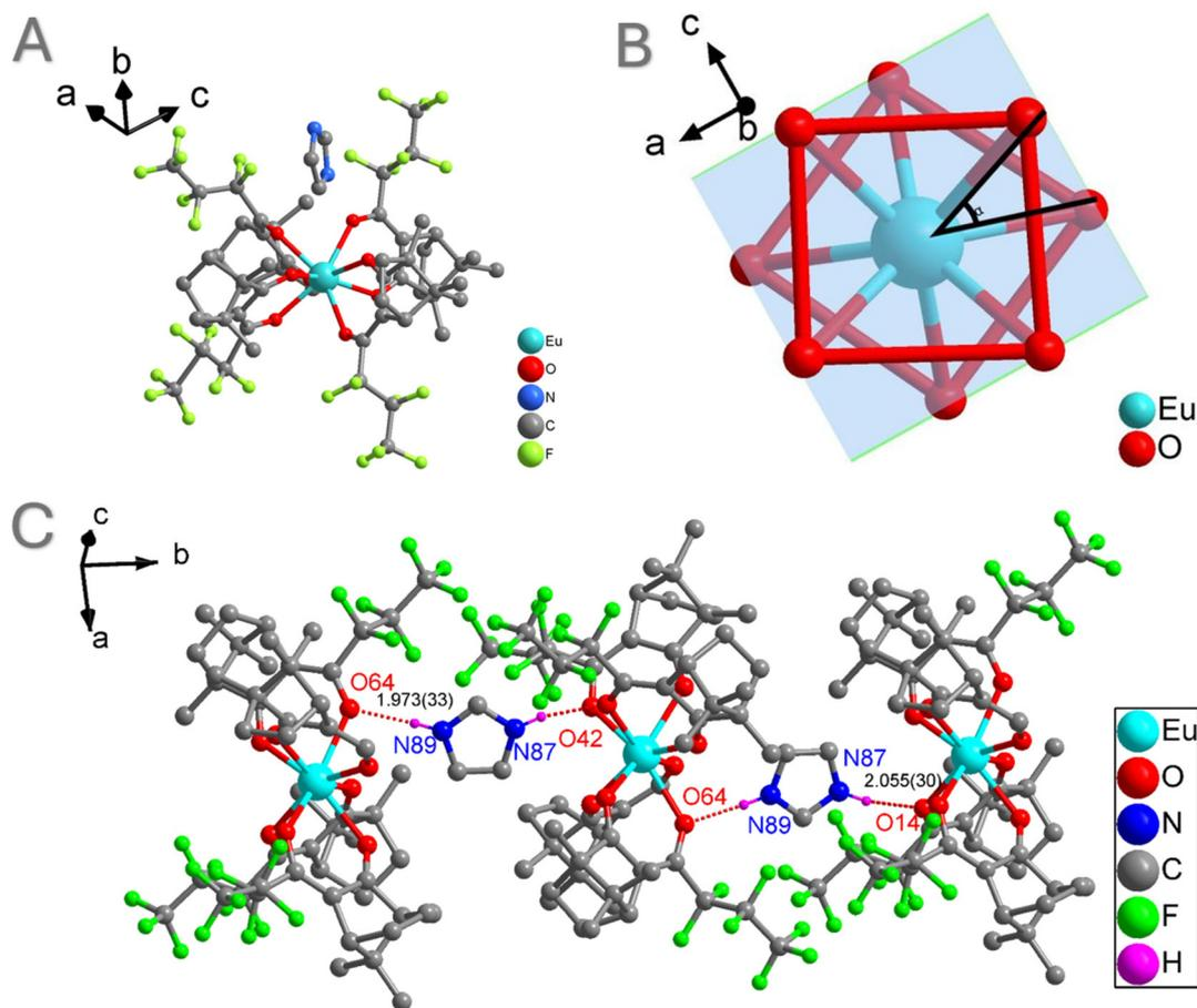
Fig. 1 (A) The asymmetric unit diagram, (B) coordination environment of the  $\text{Eu}^{3+}$  ion of complex  $\text{ImH}^+[\text{Eu}((-)\text{-hfbc})_4]^-$ , and (C) the presence of  $\text{CO}\cdots\text{HN}$  hydrogen bonds between imidazolium and oxygen atoms of the diketonate ligand.
