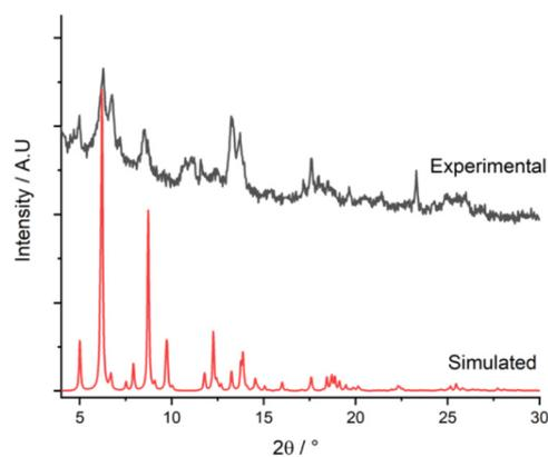
**Fig. 3** PXRD patterns for **2**. Experimental pattern (black) revealing poor crystallinity of this sample, and pattern simulated from a calculated model of a doubly interpenetrated **pcu** framework (red).
