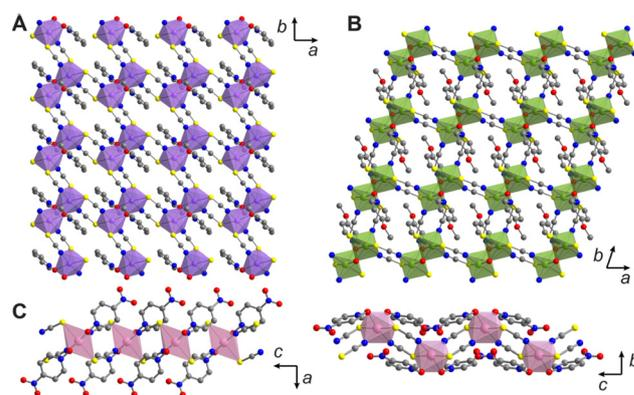
**Fig. 1** X-ray structures of 2D (A) Co(NCS)<sub>2</sub>(2-MepyO) and (B) Ni(NCS)<sub>2</sub>(4-MeOpyO), and 1D (C) Mn(NCS)<sub>2</sub>(4-NO<sub>2</sub>pyO)<sub>2</sub> (two views). Gray, blue, red, yellow, purple, green, and pink spheres are C, N, O, S, Co, Ni, and Mn, respectively. Polyhedra show connectivity.
