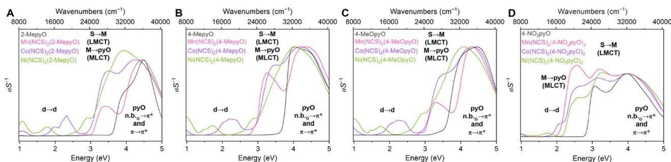
Fig. 3 UV-visible diffuse reflectance spectra as a function of metal for hybrid materials containing (A) 2-MepyO, (B) 4-MepyO, (C) 4-MeOpyO, and (D) 4- $\text{NO}_2$ pyO.
