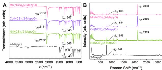
Fig. 2 (A) IR and (B) Raman spectra for  $M(\text{NCS})_2(2\text{-MepyO})$  where  $M = \text{Co}, \text{Ni},$  and  $\text{Mn}$ .
