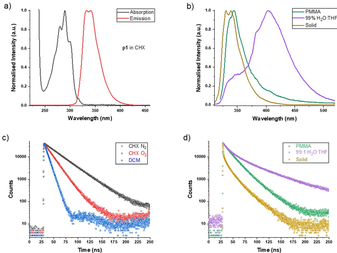
Fig. 5 Photophysical data for *C*-naphthyl-*para*-carborane **p1**. (a) Absorption and emission spectra in cyclohexane (CHX). (b) Solid state emission spectra. (c) Solution state lifetimes. (d) Solid state lifetimes.
