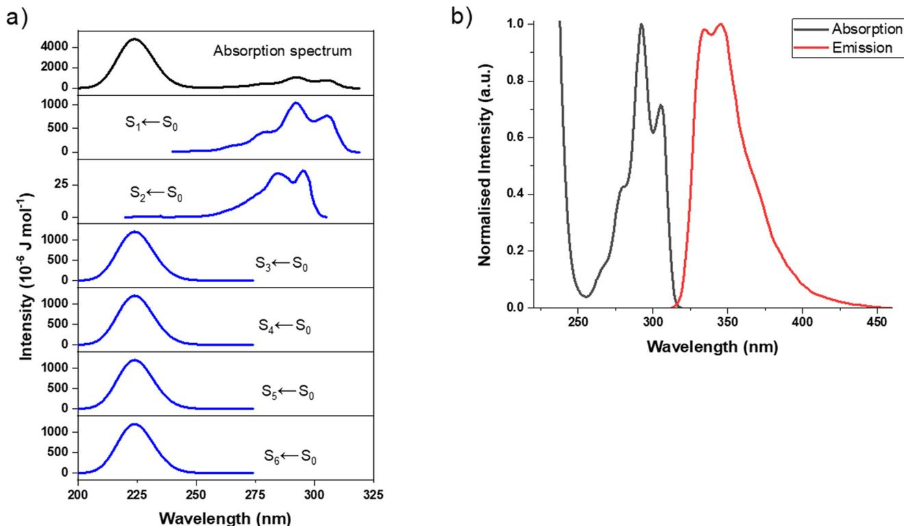
Fig. 8 (a) Calculated absorption spectrum based on combination of vibronic spectra (Adiabatic Hessian) from optimised  $S_n$  geometries with cyclohexane as solvent. (b) Simulated absorption and emission spectra for mononaphthyl-*para*-carborane **p1** from vibronic computations.
