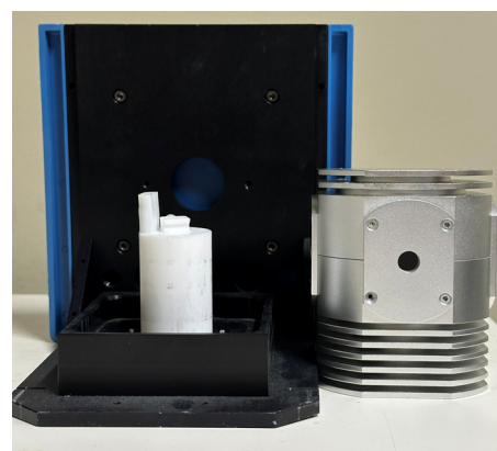
Fig. 7 Example of an integrating sphere and sample holder for absolute quantum yield measurements.
