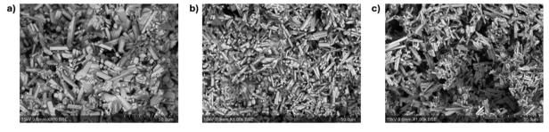
Fig. 3 Scanning electron microscopy (SEM) image of (a)  $Nb_{14}W_3O_{44}$ , (b)  $Nb_{13.5}P_{0.5}W_3O_{44}$  and (c)  $Nb_{13}PW_3O_{44}$ .
