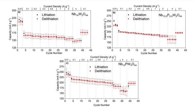
Fig. 6 Average specific capacities of (a) two  $Nb_{14}W_3O_{44}$  cells, (b) two  $Nb_{13.5}P_{0.5}W_3O_{44}$  cells and (c) two  $Nb_{13}PW_3O_{44}$  cells undergoing asymmetric cycling – such that the lithiation current density is maintained at 0.1 A g<sup>-1</sup>, while the delithiation gradually increases after 5 cycles at each rate step. The black error bars are for lithiation, the red ones are for the delithiation.
