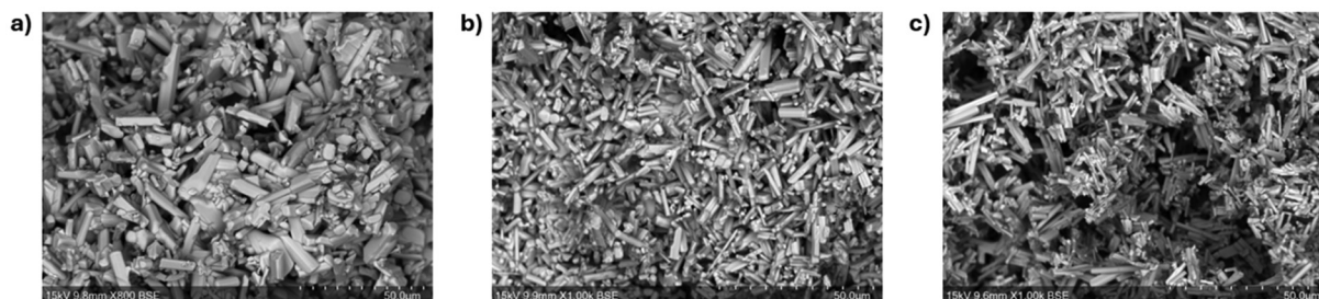
Fig. 3 Scanning electron microscopy (SEM) image of (a) \text{Nb}_{14}\text{W}_3\text{O}_{44} , (b) \text{Nb}_{13.5}\text{P}_{0.5}\text{W}_3\text{O}_{44} and (c) \text{Nb}_{13}\text{PW}_3\text{O}_{44} .
