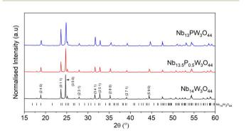
Fig. 2 PXRD patterns of Nb<sub>14</sub>W<sub>3</sub>O<sub>44</sub> (black), Nb<sub>13.5</sub>P<sub>0.5</sub>W<sub>3</sub>O<sub>44</sub> (red) and Nb<sub>13</sub>PW<sub>3</sub>O<sub>44</sub> (blue), Cu Kα, with the lattice planes shown in brackets for specific peaks. Tick marks for Nb<sub>14</sub>W<sub>3</sub>O<sub>44</sub> are shown (black ticks).
