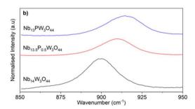
Fig. 4 Raman spectra of  $Nb_{14}W_3O_{44}$  (black),  $Nb_{13.5}P_{0.5}W_3O_{44}$  (red) and  $Nb_{13}PW_3O_{44}$  (blue) (a). Raman spectra of  $Nb_{14}W_3O_{44}$  (black),  $Nb_{13.5}P_{0.5}W_3O_{44}$  (red) and  $Nb_{13}PW_3O_{44}$  (blue) zoomed in view of the region around 900 cm<sup>-1</sup> (b).
