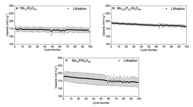
Fig. 7 Long term cycling data for duplicate cells. (a)  $Nb_{14}W_3O_{44}$ , (b)  $Nb_{13.5}P_{0.5}W_3O_{44}$  and (c)  $Nb_{13}PW_3O_{44}$ . 100 cycles were performed symmetrically at a current density of 0.6 A g<sup>-1</sup>.
