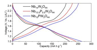
Fig. 5 Galvanostatic charge-discharge curves for the first cycle of  $Nb_{14}W_3O_{44}$  (black),  $Nb_{13.5}P_{0.5}W_3O_{44}$  (red) and  $Nb_{13}PW_3O_{44}$  (blue), vs. lithium metal, with a current density of 0.01 A g<sup>-1</sup> applied.
