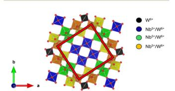
Fig. 1 Crystal structure of the NWO Wadsley-Roth material, drawn using the VESTA software.  $^{38}$  The (4  $\times$  4) block structure is highlighted by the red square. The tetrahedral sites (black tetrahedra), corner-sharing sites (blue octahedra), and edge-sharing sites (green and orange octahedra) in the structure are shown.
