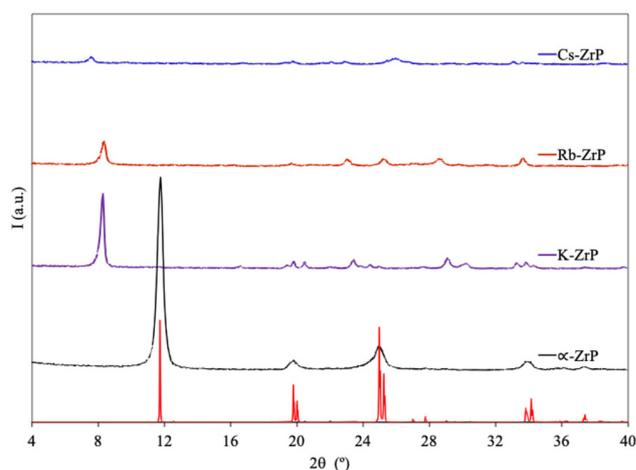
**Fig. 2** Powder X-ray diffraction patterns of the pristine  $\alpha$ -ZrP and the hydrated K-ZrP, Rb-ZrP, and Cs-ZrP phases. The red lines indicate the calculated pattern from the crystal structure of  $Zr(O_3POH)_2 \cdot H_2O$ .<sup>13</sup>
