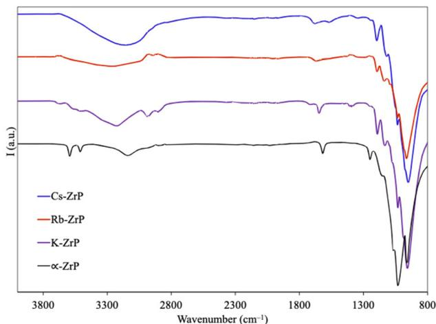
**Fig. 6** Attenuated total reflectance Fourier transform infrared analysis of the pristine  $\alpha$ -ZrP and the hydrated K-ZrP, Rb-ZrP, and Cs-ZrP phases.
