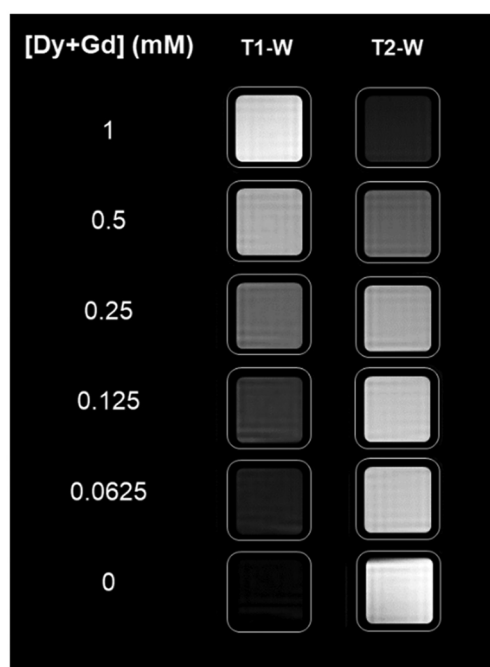
Fig. 10 Concentration-dependent T_1 - and T_2 -weighted phantom images of the \text{NaDy}_{0.44}\text{Gd}_{0.56}(\text{WO}_4)_2@PAA NPs at 3 T.
