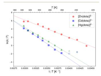
Fig. 8 Eyring plots for interconversion of two ring carbon <sup>13</sup>C NMR signals. The empty symbols represent values which significantly deviate from the linear trend and were not used for linear regression.
