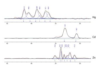
Fig. 7 The <sup>15</sup>N CP-MAS ss-NMR (71 MHz, 10 kHz) spectra of Ba(II) salts of Hg(III) (top), Cd(III) (middle) and Zn(III) (bottom) complexes. Relative integral intensities are rounded to an integer number for simplicity; the complete line fitting analysis is given in the SI. Colour codes: maroon – experimental spectra, blue – resonances of individual sites, and green – sum of the resonances of the individual sites.
