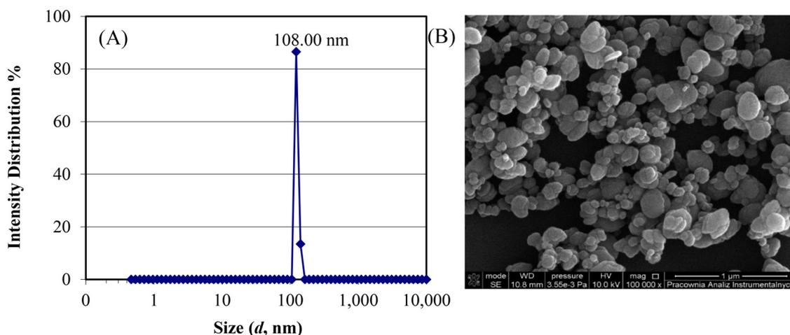
Fig. 7 Hydrodynamic size (A) and SEM image for NPs (B) of  $[\text{Ru}^{\text{III}}\text{Cl}_4(\text{Nic})_2]^-[(\text{CH}_3)_2\text{NH}_2]^+\text{DMF}_{\text{Son-10}}$  obtained from the anti-solvent method.
