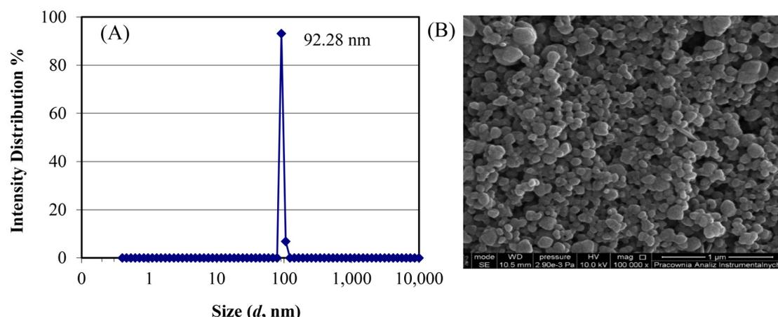
Fig. 6 Hydrodynamic size (A) and SEM image for NPs (B) of  $[\text{Ru}^{\text{III}}\text{Cl}_4(\text{Nic})_2]^-[(\text{CH}_3)_2\text{NH}_2]^+\text{DMF}_{\text{Str-10}}$  obtained from the anti-solvent method.
