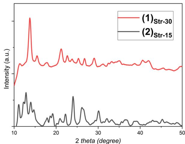
**Fig. 1** X-ray powder diffraction patterns of nanoparticles of [Ru<sup>III</sup>Cl<sub>4</sub>(Nic)<sub>2</sub>]<sup>-</sup>[(CH<sub>3</sub>)<sub>2</sub>NH<sub>2</sub>]<sup>+</sup>DMF<sub>Str-30</sub> and [Ru<sup>III</sup>Cl<sub>2</sub>(3-HPA)<sub>2</sub>]<sup>-</sup>[3-HH<sub>2</sub>PA]<sup>+</sup>(EtOH)<sub>2Str-15</sub>.
