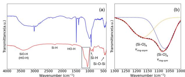
**Fig. 1** (a) FT-IR spectra of  $\text{TMA}_8(\text{Si}_8\text{O}_{20})$  (blue) and TES-Q8H8 (red). (b) Enlarged image of FT-IR spectra near  $1000\text{--}1300\text{ cm}^{-1}$  for TES-Q8H8. Orange and blue dashed lines show the fitted peaks for the asymmetric and symmetric modes of  $(\text{Si}-\text{O})_4$  rings, respectively. The black dashed line in (b) represents the combined fitting curve.
