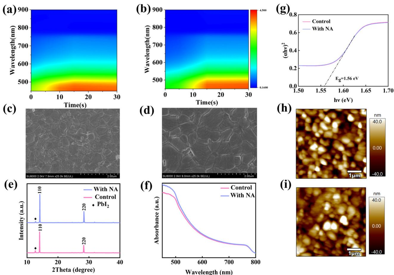
**Fig. 3** 2D UV-vis spectra of perovskite thin films prepared with (a) original and (b) NA-modified  $\text{SnO}_2$  at different annealing times. SEM images of (c)  $\text{SnO}_2/\text{PVK}$  and (d)  $\text{SnO}_2/\text{NA}/\text{PVK}$ . (e) XRD patterns, (f) UV-vis patterns, and (g) Tauc plots of perovskite thin films prepared with original and NA-modified  $\text{SnO}_2$ . AFM images of (h)  $\text{SnO}_2/\text{PVK}$  and (i)  $\text{SnO}_2/\text{NA}/\text{PVK}$ .
