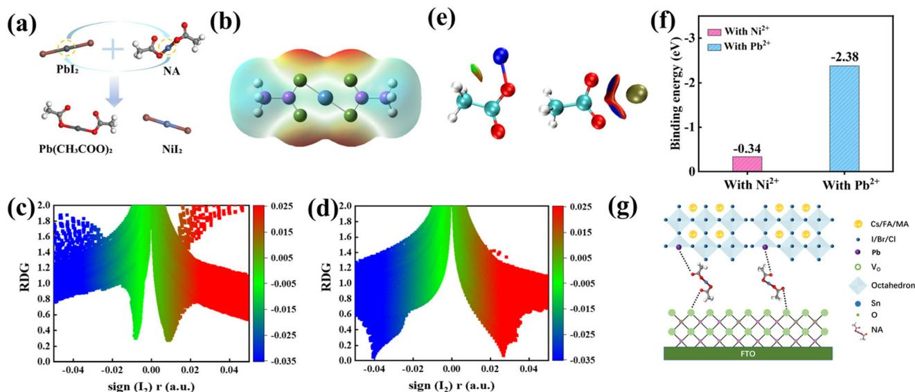
**Fig. 1** (a) Ion exchange reaction diagram. (b) Electrostatic diagram of the NA surface. Two-dimensional scatter plots of RDG for NA molecules with (c)  $\text{Ni}^{2+}$  and (d)  $\text{Pb}^{2+}$ . (e) Three-dimensional RDG isosurface diagrams of NA molecules with  $\text{Ni}^{2+}$  and  $\text{Pb}^{2+}$ . (f) Binding energy of different components. (g) Mechanism diagram.
