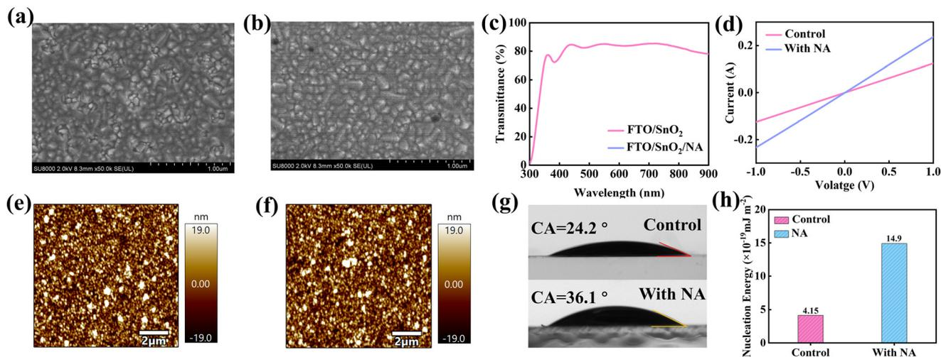
**Fig. 2** SEM images of (a) SnO<sub>2</sub> and (b) SnO<sub>2</sub>/NA. (c) Transmission spectra of different SnO<sub>2</sub> ETL thin films. (d) *I*–*V* curves of different SnO<sub>2</sub> ETL films. (e) and (f) AFM images of the SnO<sub>2</sub> film and the SnO<sub>2</sub>/NA film. The (g) water contact angle and (h) nucleation work of SnO<sub>2</sub> thin films with original and NA modification.
