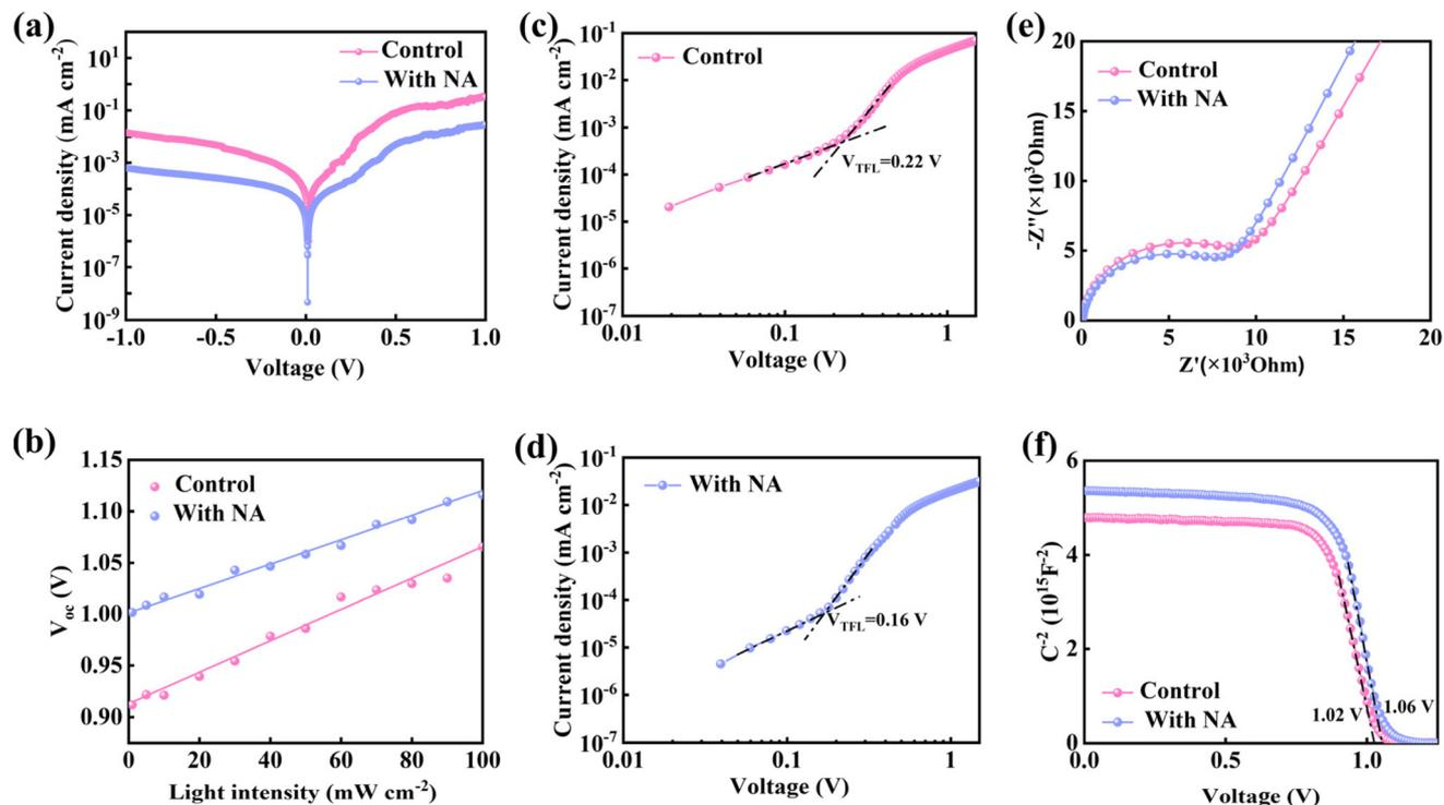
Fig. 5 (a) Dark state  $J-V$  curves of different PSCs. (b)  $V_{OC}-I$  curves and their fitting curves. (c and d)  $J-V$  curves measured by the SCLC method. (e) Nyquist curves. (f) Mott-Schottky (MS) curves.
