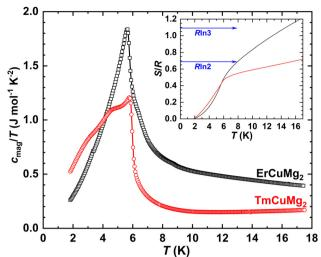
Fig. 11 Temperature dependencies of the magnetic specific heat of  $RCuMg_2$  (R = Er, Tm) obtained after the subtraction of phonon reference  $LuCuMg_2$ . Inset: Temperature evolution of the entropy near magnetic transitions
