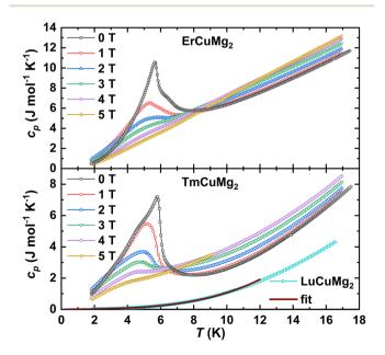
Fig. 10 Temperature dependencies of the specific heat capacities of RCuMg<sub>2</sub> (R = Er, Tm, Lu) under different magnetic fields. For LuCuMg<sub>2</sub>, the fit for the  $c_p(T) = \gamma T + \beta T^3 + \delta T^5$  ansatz is shown.
