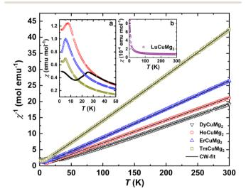
Fig. 9 Temperature dependencies of the reciprocal magnetic susceptibility  $\chi^{-1}(T)$  at  $\mu_0 H = 1$  T for RCuMg<sub>2</sub> compounds together with Curie-Weiss fits. Inset (a) magnetic susceptibility  $\chi(T)$  of RCuMq<sub>2</sub> at the antiferromagnetic transitions; (b) magnetic susceptibility  $\chi(T)$  of LuCuMg<sub>2</sub>.
