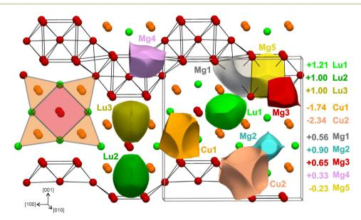
Fig. 6 Shapes and effective charges of QTAIM atomic basins for LuCuMg<sub>2</sub>. Black sticks indicate Mg–Mg contacts within the *bcc*-like slabs, while the red square and orange triangles highlight the star-like clusters.
