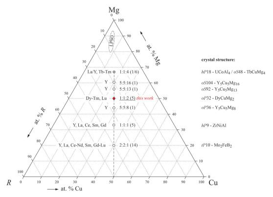
Fig. 1 Distribution and crystal structures of R-Cu-Mg compounds existing along the compositional line with a R/Cu ratio equal to 1/1. The number of representatives is indicated in parentheses. The region of existence of long-period stacking ordered (LPSO) phases known so far is also shown.
