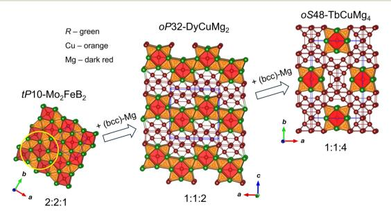
Fig. 4 Crystal structure relationships between  $R_2Cu_2Mg$ ,  $RCuMg_2$  and  $RCuMg_4$  compounds. Structures are projected along the shortest lattice vector, and unit cells are shown in blue. As a guide for the eye, one star-like cluster is highlighted by a yellow circle.
