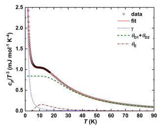
**Fig. 12** Temperature dependence of the specific heat of  $LuCuMg_2$  in the  $c_p/T$   $^3(T)$  presentation together with the fit to eqn (1) (red line) as well as separate Debye (eqn (2)), Einstein (eqn (3)) and electronic contributions.
