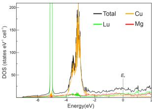
**Fig. 5** Total and species-projected electronic density of states (DOS/pDOS) for LuCuMg<sub>2</sub>.
