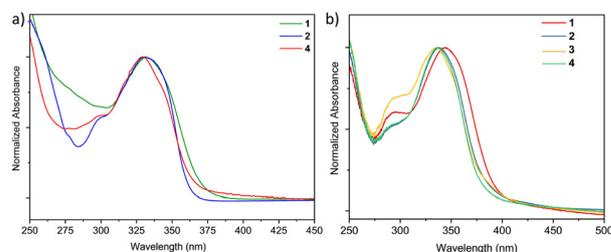
Fig. 3 UV-Vis spectra of (a) complexes **1**, **2** and **4** in DCM and (b) complexes **1–4** in a mixture of DMEM (Dulbecco's modified Eagle's medium, [+] 4.5 g L<sup>-1</sup> D-Glucose, L-Glutamin, [+] Pyruvat, Gibco™) and DMSO (dimethylsulfoxide) in a 15 : 1 ratio.
