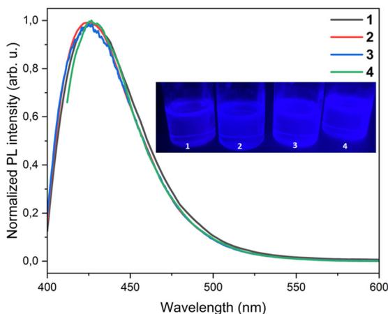
**Fig. 4** Emission spectra of the complexes 1–4 (100  $\mu\text{M}$ ) in DMSO,  $\lambda_{\text{exc}} = 365 \text{ nm}$ . Inset: photographs of DMSO solutions of complexes 1–4 when excited with 365 nm light.<sup>48</sup>
