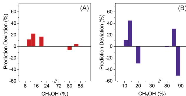
**Fig. 5** Deviations between predicted and experimentally determined values for (A) cage-type structures (%) in HSQ polymers and (B) photoluminescence quantum yield (PLQY, %) of alkyl-stabilized SiNCs synthesized from selected precursor molar ratios. In both plots, the y-axis represents the relative deviation (Predicted – Experimental)/Predicted  $\times$  100, while the x-axis corresponds to the percentages of methanol in the trichlorosilane/water/methanol reaction mixture.
