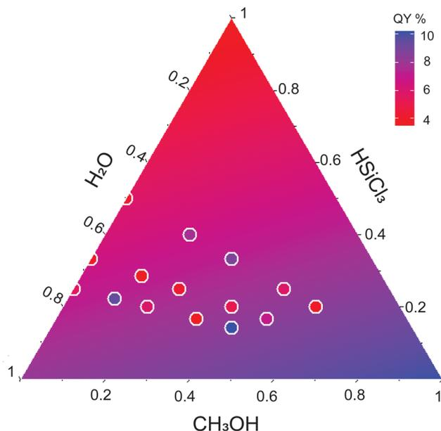
**Fig. 4** Prediction of PLQY (%) values of alkyl-stabilized SiNCs with RSM using precursor molar ratios as input variables. The colored circles represent the experimental data used to fit Scheffé's polynomial model.
