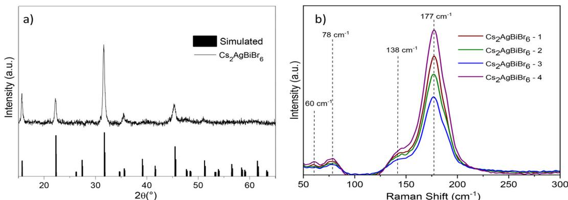
Fig. 1 (a) X-ray diffraction pattern and (b) Raman spectra of Cs<sub>2</sub>AgBiBr<sub>6</sub> nanocrystals.
