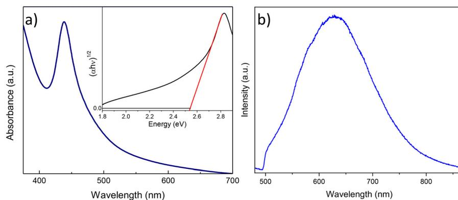
Fig. 3 (a) The UV-Vis absorption spectrum, Tauc plot (inset), and (b) photoluminescence (PL) spectrum of  $\text{Cs}_2\text{AgBiBr}_6$  nanocrystals.
