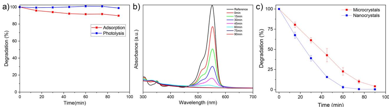
**Fig. 4** (a) Photolysis and adsorption behaviour of rhodamine B; (b) UV-Vis absorption spectra of RhB as a function of irradiation time; and (c) comparative photocatalytic activity of  $\text{Cs}_2\text{AgBiBr}_6$  nanocrystals and microcrystals; the experiments were performed in triplicate, and the error bars represent the standard deviation.
