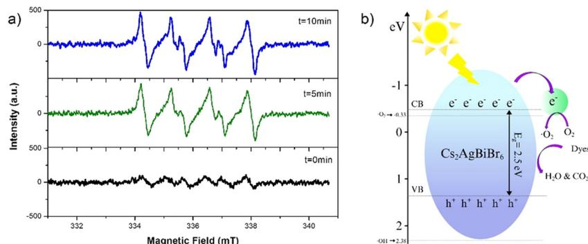
**Fig. 5** (a) Electron Spin Resonance (EPR) measurements; (b) proposed pathway for dye degradation, dominated by  $\cdot\text{O}_2^-$  radicals.
