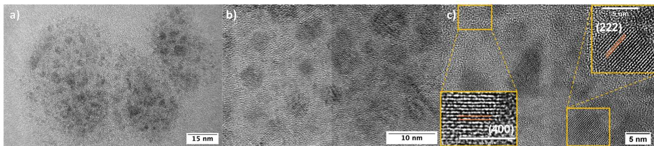
Fig. 2 (a–c) Transmission Electron Microscopy (TEM) images of  $\text{Cs}_2\text{AgBiBr}_6$  nanocrystals at increasing magnifications, (c) shows lattice fringes of two particles: the left one has a spacing of 2.82 Å (400) and the right one, 3.28 Å (222).
