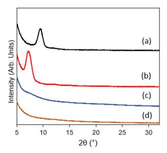
**Fig. 8** X-ray diffractograms of (a) Et-DTOA, (b) nPr-DTOA, (c) iPr-DTOA, and (d) nBu-DTOA based Cu-R DTOA thin films deposited on Si substrates.
