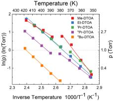
Fig. 5 TGA and vapor pressure plots of DTOA and compounds 1-5.
