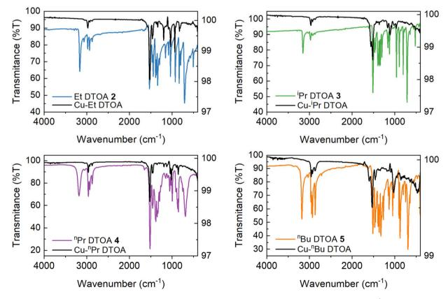
Fig. 7 FTIR of DTOA derivative 2-5 and their respective hybrid films. The horizontal axis represents wavenumber (cm<sup>-1</sup>) and the vertical axis represents transmittance (%). The left vertical scale corresponds to the organic precursors, while the right vertical scale corresponds to the hybrid thin films.
