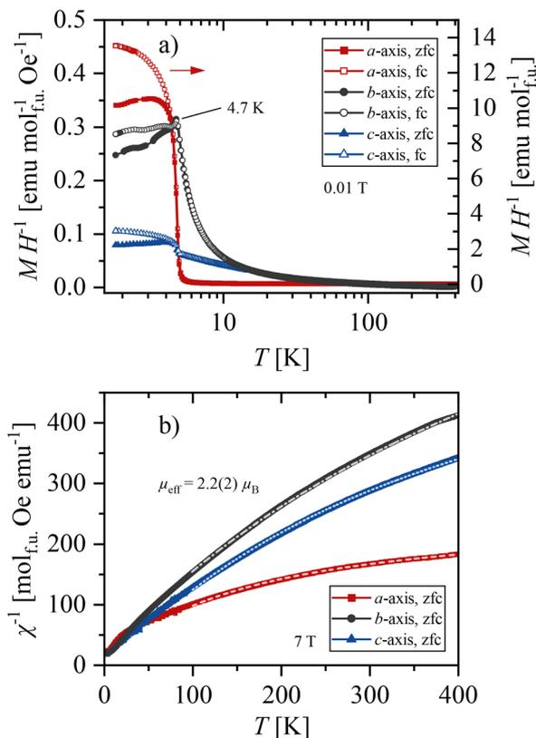
**Fig. 4** (a) Temperature-dependent susceptibility and (b) inverse susceptibility of CeFeSb<sub>3</sub>, broken lines represent the modified Curie–Weiss fits.
