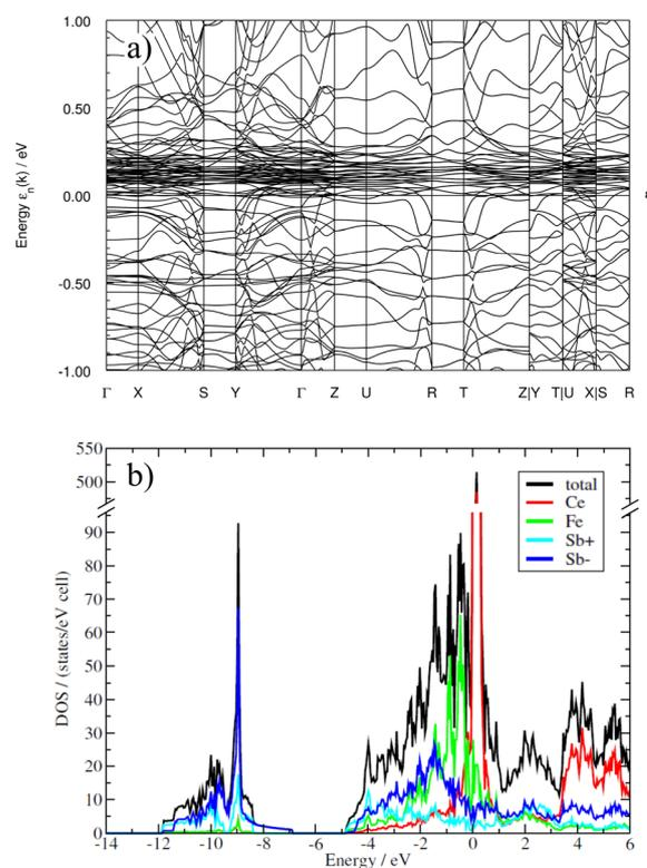
**Fig. 2** (a) Calculated band structure and (b) density of states (DOS) of CeFeSb<sub>3</sub>. The large dispersion of states close to the Fermi level reflects its strong metallic nature; Sb+ and Sb– denote Sb atoms with positive and negative partial charges, respectively.
