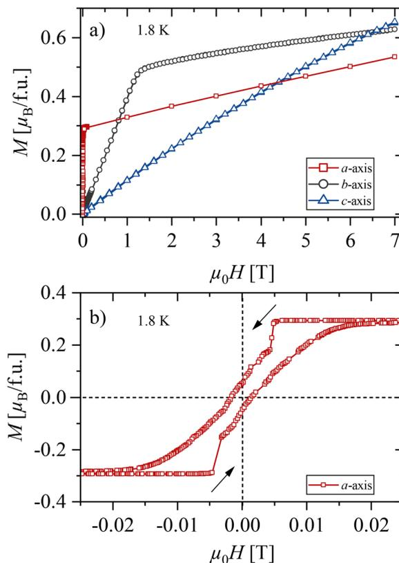
**Fig. 5** (a) Field-dependent magnetisation of CeFeSb<sub>3</sub> at  $T = 1.8$  K for the three crystallographic directions, (b) field-dependent magnetisation at  $T = 1.8$  K with the magnetic field applied parallel to the *a*-axis revealing hysteretic behaviour at small fields.
