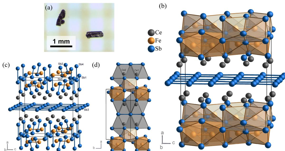
**Fig. 1** (a) Flux-grown CeFeSb<sub>3</sub> crystals. (b) Crystal structure of CeFeSb<sub>3</sub> approximately along the [010] direction with FeSb<sub>6</sub> octahedra and Sb(3) plane. (c) Fe–Fe and shortest Sb–Sb distances shown in a ball-and-stick representation; see text for details. (d) Crystal structure along the [001] direction, revealing the two crystallographically inequivalent Ce sites.
