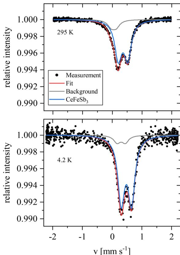
**Fig. 8**  $^{57}\text{Fe}$ -Mössbauer spectra of  $\text{CeFeSb}_3$  at 295 K and 4.2 K, indicating non-magnetic behaviour of the Fe atoms. The background signal primarily originates from steel components of the cryostat employed in the measurements. Additionally, a minor contribution from  $\text{FeSb}$  may be present as evidenced by Rietveld refinement (Fig. S1, ESI†).
