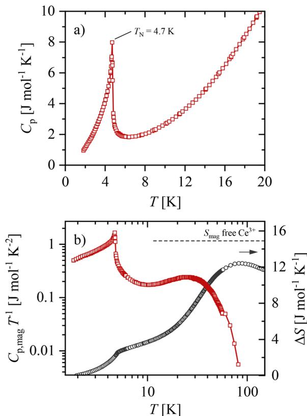
Fig. 7 (a) Temperature-dependence of the specific heat and (b) temperature-dependence of the magnetic contribution of the specific heat divided by temperature and released magnetic entropy of CeFeSb<sub>3</sub> at zero magnetic field.
