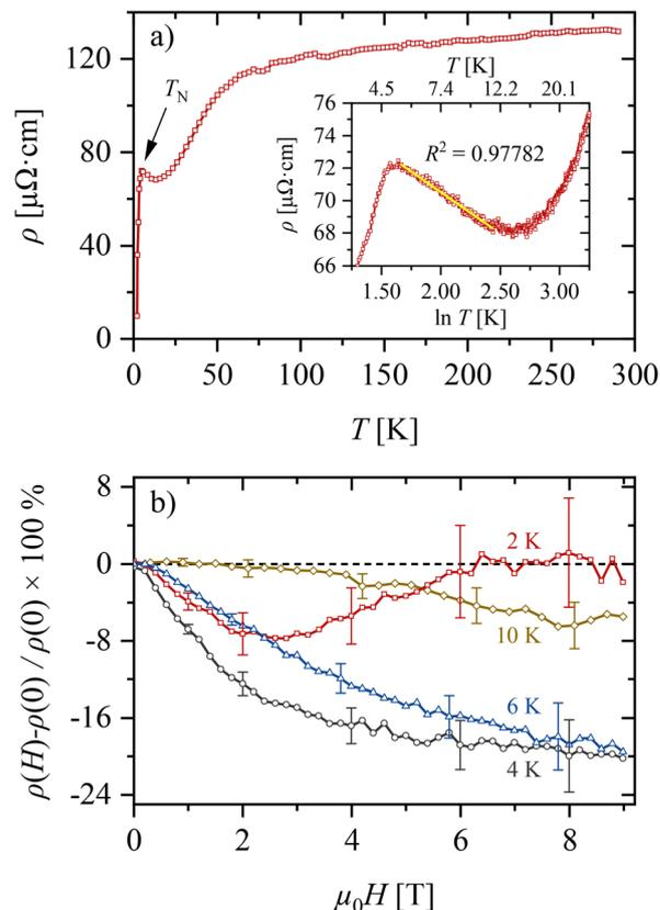
**Fig. 9** (a) Temperature-dependent resistivity and (b) magnetoresistance of  $\text{CeFeSb}_3$  with the electric current and magnetic field applied parallel to the  $bc$ -plane and the  $a$ -axis, respectively.
