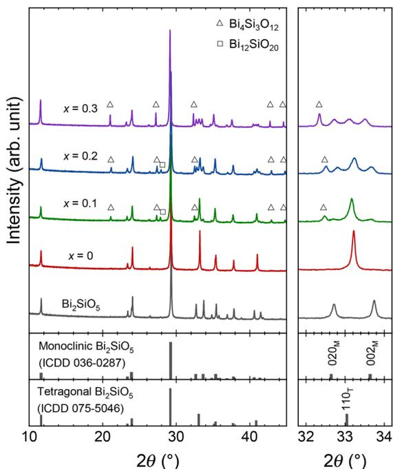
**Fig. 2** XRD patterns of the  $(\text{Bi}_{0.97}\text{La}_{0.03})_2\text{Si}_{1-x}\text{Ge}_x\text{O}_5$  ceramics with  $x = 0, 0.1, 0.2, \text{ and } 0.3$ , as well as a pristine  $\text{Bi}_2\text{SiO}_5$  ceramic. (Bottom panel) Reference patterns of monoclinic and tetragonal  $\text{Bi}_2\text{SiO}_5$ .
