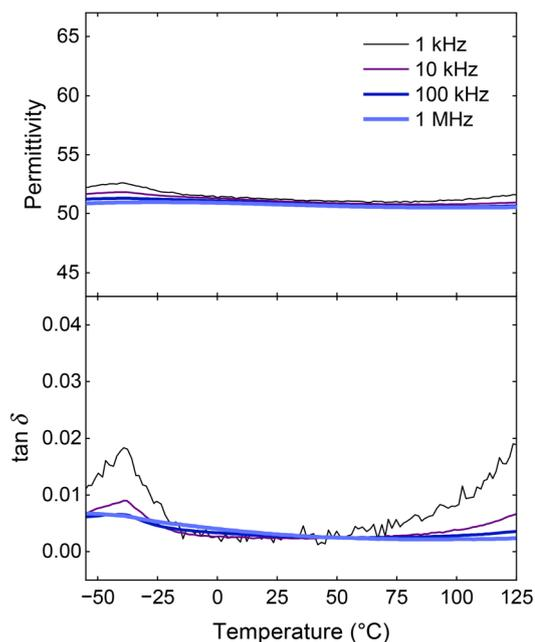
**Fig. 7** Temperature dependences of the dielectric permittivity (top panel) and dielectric loss (bottom panel) for  $(\text{Bi}_{0.97}\text{La}_{0.03})_2\text{Si}_{0.8}\text{Ge}_{0.2}\text{O}_5$ , measured at 1 kHz–1 MHz.
