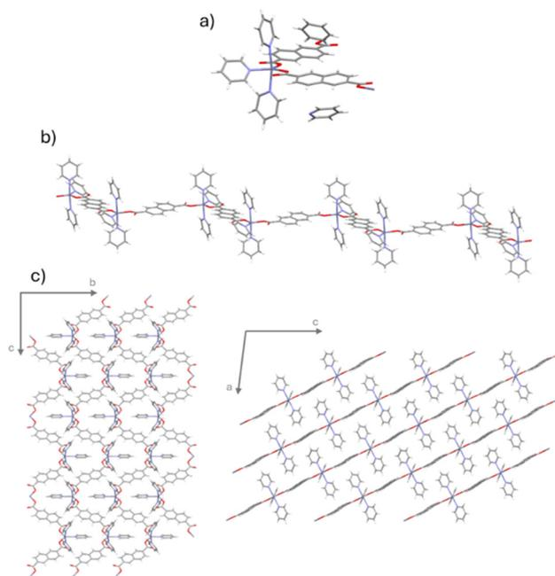
**Fig. 6** (a) Asymmetric unit of **PUM210\_PY** obtained by degradation of **PUM210@DMF** in pyridine. (b) Visualization of the mono-dimensional chain of the polymer and (c) visualization of the packing of the chains along the crystallographic axis *a* (left) and *b* (right), respectively. The included molecules of pyridine are not reported for clarity.
