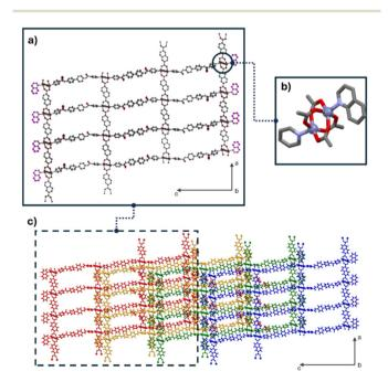
Fig. 7 (a) Visualization of a single frame of PUM210@(quino)1, highlighting the coordinated quinoline in magenta. (b) View of the SBU of PUM210@(quino)<sub>1</sub> showing the coordinated molecule of quinoline occupying the apical position of the Zn atom. (c) Polycatenation displayed by PUM210@(quino)<sub>1</sub>, similar to that of the PUM210@DMF.<sup>39</sup>
