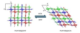
Fig. 3 Representation of the two frameworks of PUM168@DMF (pristine) and PUM168@ACN (after DMF-to-ACN exchange).
