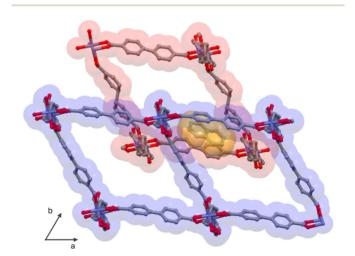
Fig. 4 Visualization of the quinoline molecule (colored in yellow) trapped in the distorted squares defined by the dicarboxylate linkers in the framework of PUM168@(quino)<sub>1</sub>.
