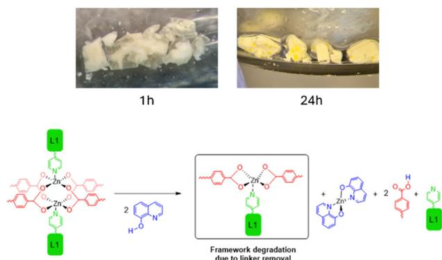
**Fig. 5** Top-left: Opacification of the crystals of **PUM168@ACN** after soaking in a 0.1 M acetonitrile solution of 8-hydroxyquinoline. Top-right: appearance of the new crystalline phase corresponding to  $\text{Zn}(\text{8-O-QUI})_2$  on the surface of the damaged MOF crystals. Bottom: simplified reaction scheme.
