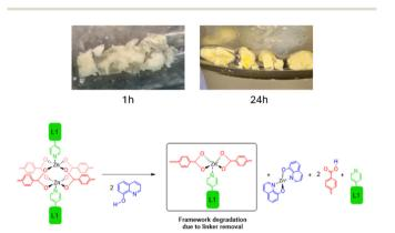
Fig. 5 Top-left: Opacification of the crystals of PUM168@ACN after soaking in a 0.1 M acetonitrile solution of 8-hydroxyquinoline. Topright: appearance of the new crystalline phase corresponding to Zn(8-O-QUI)<sub>2</sub> on the surface of the damaged MOF crystals. Bottom: simplified reaction scheme.
