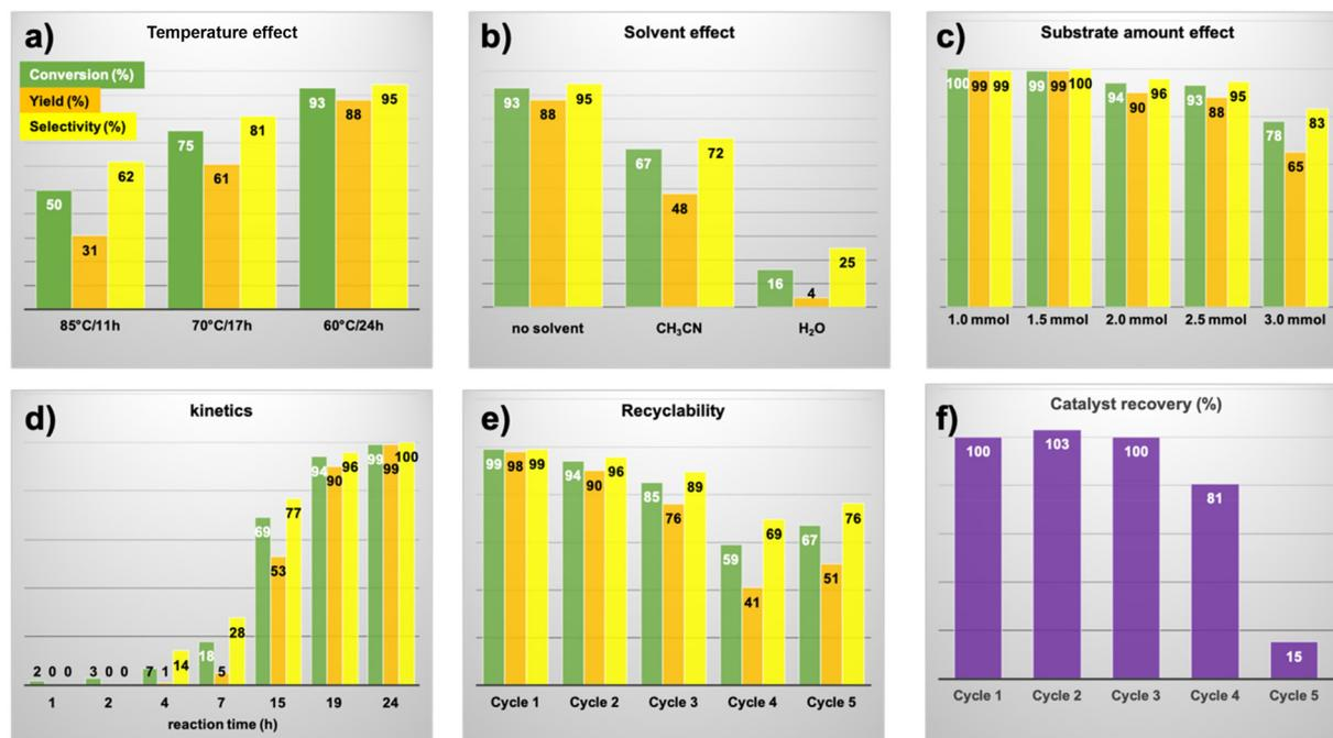
Fig. 7 Oxidation of benzyl alcohol to benzoic acid with  $\{\text{PV}^{\text{IV}}\text{W}_{11}\}^{5-}@CD\text{-EPI}$  using  $t\text{-BuOOH}$  as the oxidizing agent: (a) temperature effect, (b) solvent effect, (c) substrate amount effect, (d) kinetic study, and (e and f) recyclability study. Reaction conditions when not indicated: 2.5 mmol substrate in (a) and (b) or 1.5 mmol substrate in (d)–(f), 12.5 mmol oxidizing agent, 0.01 mmol POM, 1 mL solvent, 60 °C, 24 h.
