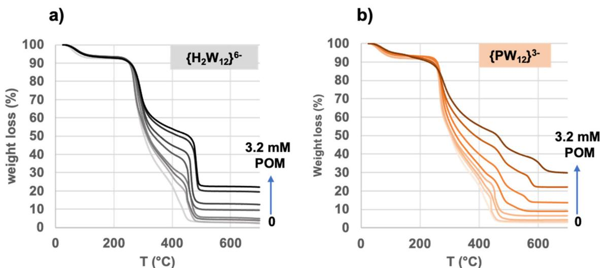
**Fig. 4** TGA curves of POM@CD-EPI composites obtained upon adsorption of 5 mL of (a)  $[\text{H}_2\text{W}_{12}\text{O}_{40}]^{6-}$  or (b)  $[\text{PW}_{12}\text{O}_{40}]^{3-}$  solutions of varied concentrations on 75 mg of insoluble polymer CD-EPI(25). Experimental conditions: CD polymer amount = 75 mg, POM volume = 5 mL, POM concentration = 0–3.2 mM, contact time = 60 min, stirring speed = 500 rpm, pH = 1, and temperature = 25 °C.
