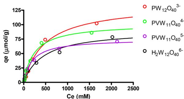
**Fig. 5** Langmuir isotherm curves for the adsorption of  $[\text{PW}_{12}\text{O}_{40}]^{3-}$ ,  $[\text{PV}^{\text{IV}}\text{W}_{11}\text{O}_{40}]^{4-}$ ,  $[\text{PV}^{\text{V}}\text{W}_{11}\text{O}_{40}]^{5-}$ , and  $[\text{H}_2\text{W}_{12}\text{O}_{40}]^{6-}$  on insoluble polymer CD–EPI(25). Experimental conditions: CD polymer amount = 75 mg, POM volume = 5 mL, POM concentration = 0–3.2 mM, contact time = 60 min, stirring speed = 500 rpm, pH = 1, and temperature = 25 °C.
