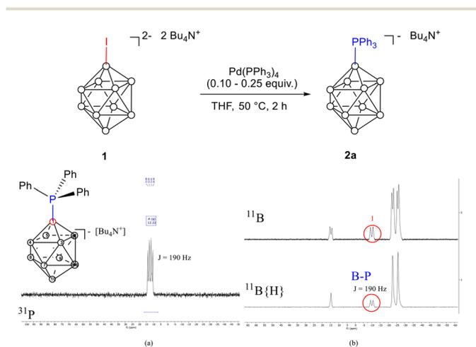
**Scheme 1** Preparation of  $[\text{N}(n\text{-C}_4\text{H}_9)_4][1\text{-B}_{10}\text{H}_9(\text{PPh}_3)]$  **2a**. (a)  $^{31}\text{P}$  NMR spectrum for  $[\text{B}_{10}\text{H}_9\text{PR}_3][\text{N}(n\text{-C}_4\text{H}_9)_4]$  **2a** and (b)  $^{11}\text{B}$  NMR and  $^{11}\text{B}\{^1\text{H}\}$  spectra for  $[\text{B}_{10}\text{H}_9\text{PPh}_3][\text{N}(n\text{-C}_4\text{H}_9)_4]$  **2a**.
