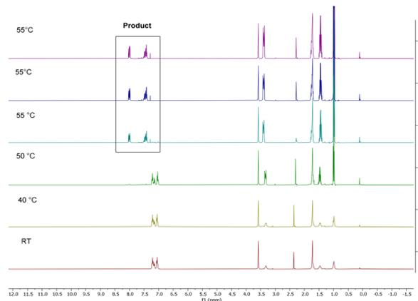
**Fig. 2** <sup>1</sup>H NMR spectra for the reaction mixture between [N(*n*-C<sub>4</sub>H<sub>9</sub>)<sub>4</sub>]<sub>2</sub>[B<sub>10</sub>H<sub>9</sub>I] and Pd(PPh<sub>3</sub>)<sub>4</sub> in d<sup>8</sup>-THF after 15 min at RT, 313 K (40 °C), 323 K (50 °C) and 328 K (55 °C).
