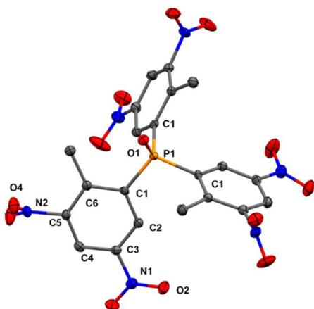
**Fig. 3** Solid-state structure of **2Me**. The asymmetric unit is composed of 1/3 of the molecule. The compound crystallizes with one (disordered) dichloromethane molecule per  $\text{Ar}_3\text{P}=\text{O}$  molecule (not shown, see ESI†). Hydrogen atoms were omitted for clarity. Selected parameters: bond distances (Å) P1–C1 1.820(3), P1–O1 1.488(4); bond angles (°) C1–P1–C1 105.4(1); torsion angles (°) O2–N1–C3–C2 11.3(5), O4–N2–C5–C6 –61.1(5).
