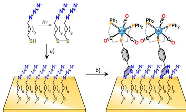
**Scheme 3** Two step surface functionalization of Au(111) with **8**. Preparation of N<sub>3</sub>-terminated Au(111) surface with 5 mM N<sub>3</sub>SH (abs. EtOH) for 48 h (a). Covalent attachment of **8** *via* CuAAC for 2 h, rt, inert-atm (b).
