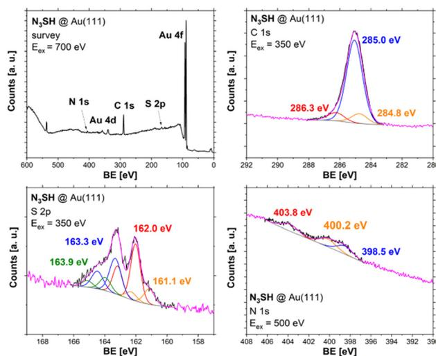
**Fig. 5** XPS spectra of an Au(111)-surface functionalized with a **N<sub>3</sub>SH**-SAM. Survey (top left), C 1s- (top right), S 2p- (bottom left) and N 1s- region (bottom left). For fitting parameters see Table S9<sup>†</sup>
