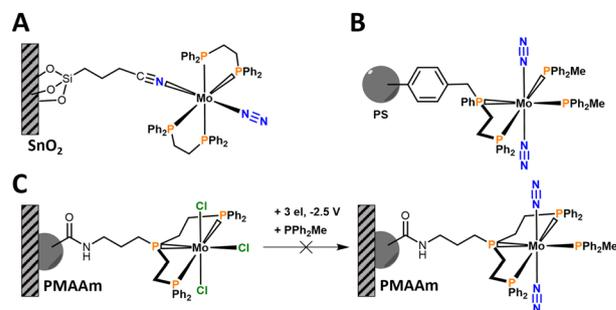
**Scheme 1** Schematic depiction of immobilized N<sub>2</sub>-complexes onto electrode surfaces or polymers making use of SnO<sub>2</sub>- (A) or polystyrene-coated electrodes (B) or polymethacrylamide functionalized polymers (C).<sup>21–23</sup>
