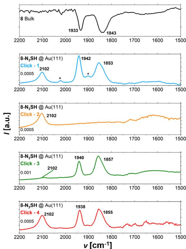
**Fig. 6** Bulk IR of **8** and IRRA spectra of **8-N<sub>3</sub>SH@Au(111)** prepared employing protocols **Click 1–4** in the CO-stretch region. The visible feature at 2102 cm<sup>-1</sup> corresponds to unfunctionalized azides of the SAM backbone. \* mark small portions of *mer-8*. For full spectrum see Fig. S57.†
