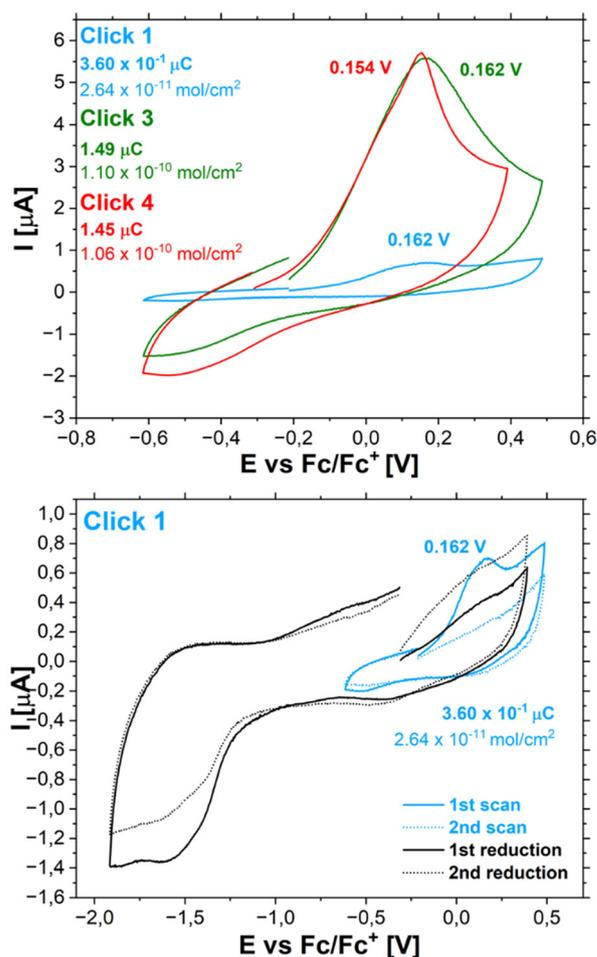
**Fig. 9** Top: CVs of  $8\text{-N}_3\text{SH@Au-WE}$  prepared with the Click 1 and Click 3, 4 protocols (1<sup>st</sup> experimental scan). Bottom: CVs of the 1<sup>st</sup> and 2<sup>nd</sup> oxidative scan (turquoise) in the redox-active region of **8**. Subsequent reductive scans (black) show a very broad reductive wave around  $-1.5$  V corresponding the Au–S cleavage. Experimental data for Click 3 and Click 4 see Fig. S65–S67.<sup>†</sup>
