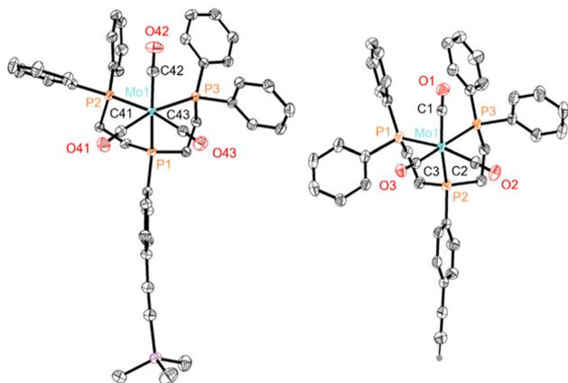
**Fig. 2** Crystal structures of [Mo(CO)<sub>3</sub>(etPP<sup>PhTMS</sup>P)] **7** (left) and [Mo(CO)<sub>3</sub>(etPP<sup>PhH</sup>P)] **8** (right) shown as thermal ellipsoids with 70% probability. Please note that for both compounds only one of the two crystallographically independent complexes are shown. C is gray, P is orange, Mo is turquoise, O is red, Si is purple and all H atoms except for the C≡C–H moiety are omitted for clarity.
