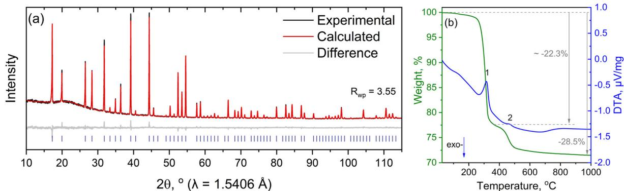
**Fig. 3** XRPD pattern with Rietveld fit (a) and TG-DTA curves (b) of pure katoite prepared by hydration of tricalcium aluminate ( $\text{Ca}_3\text{Al}_2\text{O}_6$ ) under hydrothermal conditions.
