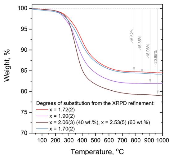
Fig. 7 TGA curves of four hydrogrossular samples corresponding to those described in Table 1.
