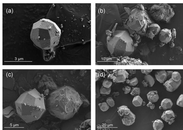
**Fig. 2** SEM micrographs of katoite prepared by the hydration of tricalcium aluminate ( $\text{Ca}_3\text{Al}_2\text{O}_6$ ) under hydrothermal conditions. Panels (a)–(d) show different magnifications (as shown by scale bars).
