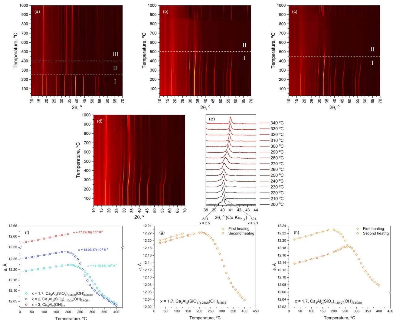
**Fig. 8** VT-XRPD plots of pure katoite (a), hydrogrossular samples with  $x = 1.72$  (b) and  $1.90$  (c) and a two-phase sample with  $x = 2.06$  and  $2.53$  (d) from Table 2. Evolution of 521 peaks in 2-phase hydrogrossular samples upon heating (e); evolution of the unit cell parameter from the samples with  $x = 1.72$  and  $1.90$  (f); the sample with  $x = 1.72$  before and after pre-heating to  $125$  °C (g); the sample with  $x = 1.70$  before and after pre-heating to  $260$  °C (h).
