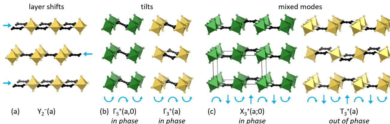
**Fig. 3** Examples of rigid-unit distortions in Hofmann complexes: (a) layer shifts, (b) tilts, and (c) mixed tilt–shift modes. The irrep, order parameter direction and correlation along  $c$  (vertical, in phase/out of phase) are given for each distortion. Structures with the  $P4/mmm$  and  $Ammm$  parents are shown in green and yellow, respectively.
