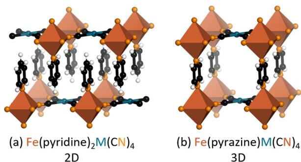
Fig. 1 (a) 2D  $\text{Fe}(\text{pyridine})_2\text{M}(\text{CN})_4$ ,<sup>25</sup> and (b) 3D  $\text{Fe}(\text{pyrazine})\text{M}(\text{CN})_4$ .<sup>26</sup> Fe is shown in brown, N in orange, C in black, H in white, and M in dark blue. Linker disorder has been removed for clarity.
