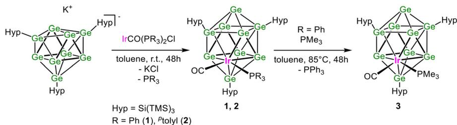
**Scheme 1** Reaction of  $K[Hyp_3Ge_9]$  with  $Ir(CO)(PR_3)_2Cl$  in toluene, yielding  $[Hyp_3Ge_9Ir(CO)(PR_3)]$ ,  $R = Ph$  (1),  $p\text{-tolyl}$  (2), and follow-up reaction of 1 with  $PMe_3$ , yielding  $[Hyp_3Ge_9Ir(CO)(PMe_3)]$  (3).
