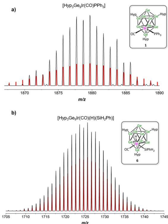
**Fig. 2** LIFDI mass spectra of (a) [Hyp<sub>3</sub>Ge<sub>9</sub>Ir(CO)(PPh<sub>3</sub>)] (1) and (b) [Hyp<sub>3</sub>Ge<sub>9</sub>Ir(CO)(H)(SiH<sub>2</sub>Ph)] (6). Experimental spectra and simulated isotope pattern are shown in black and red, respectively.
