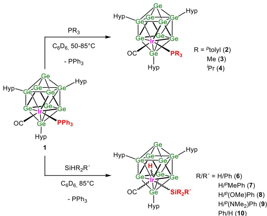
**Scheme 2** Reaction schemes for (top) the phosphine exchange reactions between 1 and  $PR_3$  ( $R = p\text{-tolyl}$ , Me,  $i\text{-Pr}$ ) and (bottom) the Si–H bond activation of  $SiHR_2R'$  [ $R/R' = H/Ph$ ,  $H^i/MePh$ ,  $H^i/(OMe)Ph$ ,  $H^i/(NMe_2)Ph$ , Ph/H] with 1.
