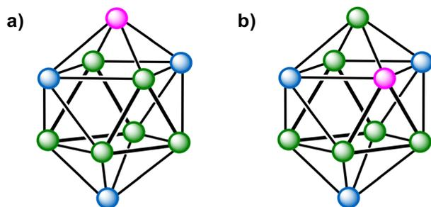
**Fig. 1** Incorporation of transition metal atoms into  $[E_9]^{4-}$  ( $E = Si-Pb$ ) cluster cores forming ten atomic cluster species: (a)  $\eta^4$ -capping the open square of the antiprism and (b)  $\eta^5$ -coordination (as part of the square). Green spheres indicate tetrel element atoms, blue spheres indicate either a tetrel element atom or a Ge-silyl group, and pink spheres represent transition metal atoms with ligands.
