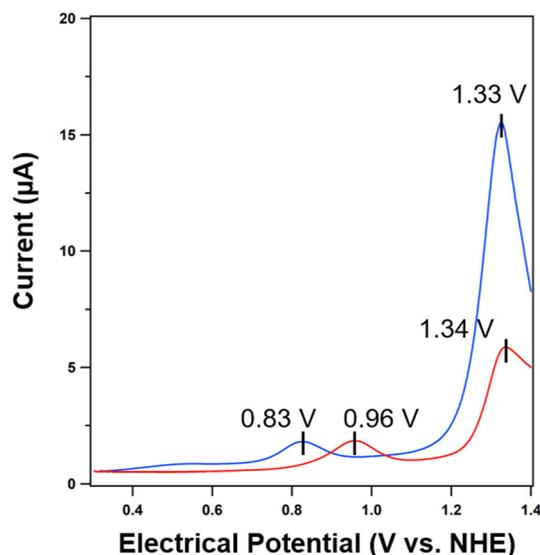
Fig. 4 SWV traces of **1a** (blue) and the mixture of **2-syn** and **2-anti** (red) (0.1 mM) in B-R buffer at pH 8.0 at 298 K, using a 3 mm GC working electrode (0.07 cm<sup>2</sup>), Pt wire counter electrode, Ag/AgCl reference electrode, potential increase: 0.001 V, amplitude: 0.025 A, frequency: 10 Hz, and sensitivity: 10 mAV<sup>-1</sup>.
