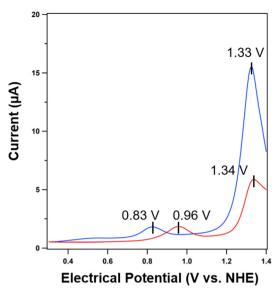
Fig. 4 SWV traces of 1a (blue) and the mixture of 2-syn and 2-anti (red) (0.1 mM) in B–R buffer at pH 8.0 at 298 K, using a 3 mm GC working electrode (0.07 cm $^2$ ), Pt wire counter electrode, Ag/AgCl reference electrode, potential increase: 0.001 V, amplitude: 0.025 A, frequency: 10 Hz, and sensitivity: 10 mAV $^{-1}$ .
