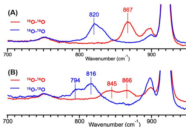
Fig. 3 Resonance Raman spectra of **1a** (A) and a mixture of **2-syn** and **2-anti** (B) in MeCN at -30 °C with excitation at 405 nm. The spectra of <sup>16</sup>O-<sup>16</sup>O and <sup>18</sup>O-<sup>18</sup>O complexes are shown as red and blue lines, respectively.
