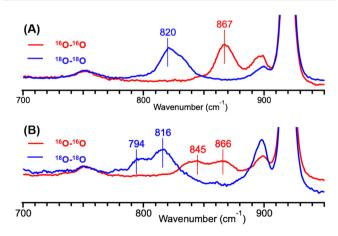
Fig. 3 Resonance Raman spectra of 1a (A) and a mixture of 2-syn and 2-anti (B) in MeCN at -30 °C with excitation at 405 nm. The spectra of  $^{16}O-^{16}O$  and  $^{18}O-^{18}O$  complexes are shown as red and blue lines, respectively.
