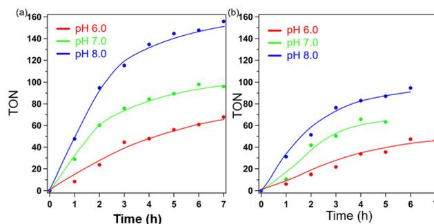
Fig. 6 The controlled potential electrolysis of **1a** (a) and a mixture of **2-syn** and **2-anti** (b) (0.1 mM) was carried out at 1.4 V (vs. NHE) in B-R buffer at pH 6.0, 7.0, and 8.0. Conditions: working electrode Pt mesh, counter electrode Pt wire, reference electrode Ag/AgCl. The amount of O<sub>2</sub> evolution in the CPE was determined by GC analysis.
