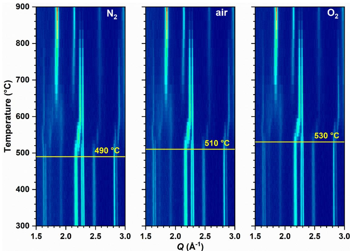
Fig. 6 Contour plots of the *in situ* XRD patterns obtained for the thermal decomposition of  $\text{La}_4\text{Ni}_3\text{O}_{8.4}\text{F}_{3.5}$  in different atmospheres. The start of the decomposition is highlighted by a yellow line in each plot.
