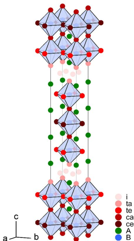
**Fig. 1** Representation of the ideal  $n = 3$  Ruddlesden–Popper structure (space group:  $I4/mmm$ ). The  $\text{BO}_6$  octahedra are shown and the different anion sites are indicated by different shades of red.
