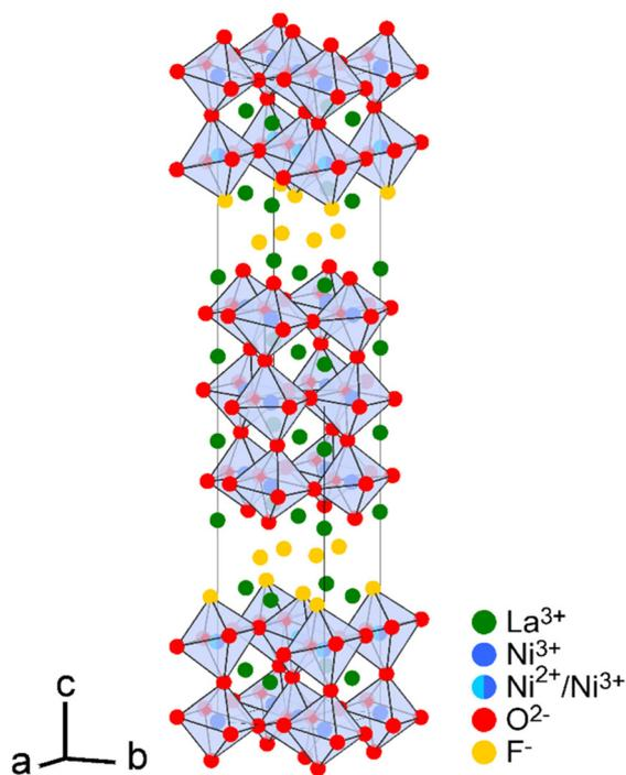
Fig. 5 Crystal structure of La<sub>4</sub>Ni<sub>3</sub>O<sub>8.4</sub>F<sub>3.5</sub> (space group: P2<sub>1</sub>/a) with representation of Ni-coordination polyhedra.
