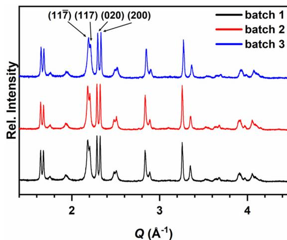
Fig. 3 XRD patterns of La<sub>4</sub>Ni<sub>3</sub>O<sub>8.4</sub>F<sub>3.5</sub> from different batches. The indices are given for the (117)/(11-7) and (200)/(020) reflexes, indicating the difference in reflection broadening.
