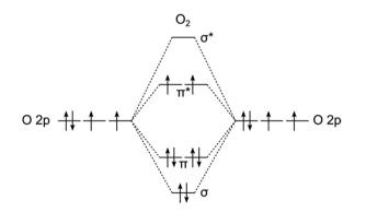
Fig. 1 Simplified O<sub>2</sub> molecular orbital diagram considering only the O 2p states.
