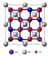
Fig. 3 Spinel crystal structure shown for the example of NiCo<sub>2</sub>O<sub>4</sub>.
