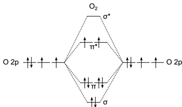
Fig. 1 Simplified O<sub>2</sub> molecular orbital diagram considering only the O 2p states.
