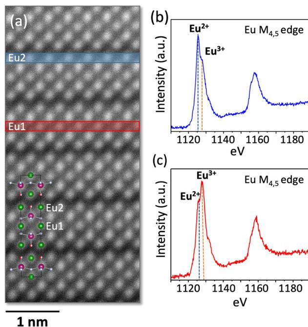
Fig. 5 (a) HAADF-STEM image of the  $\text{Eu}_3\text{Ta}_2\text{ON}_5$  crystal along the [010] zone axis with the  $\text{Eu}_3\text{Ta}_2\text{ON}_5$  structure overlay (Eu: green, Ta: magenta, O: red and N: light gray). (b) and (c) show the averaged EEL M4,5 spectra obtained from Eu2 and Eu1 sites of the  $\text{Eu}_3\text{Ta}_2\text{ON}_5$  structure, marked in blue and red in (a), respectively.
