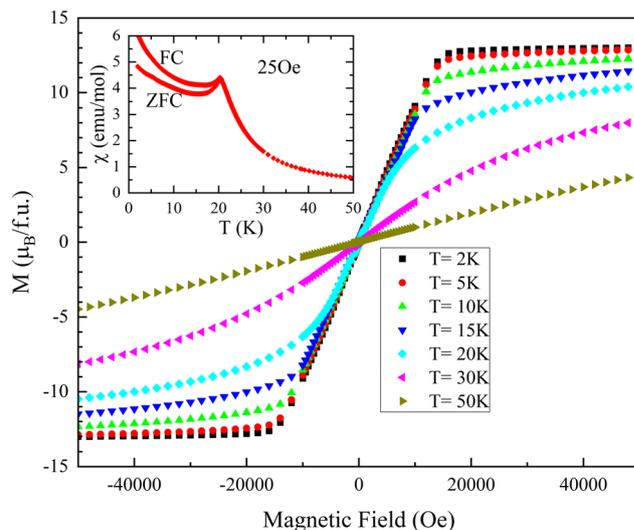
Fig. 7 Magnetization loops recorded at several temperatures (indicated) up to  $\pm 5$  T. Inset: zero field-cooled/field-cooled magnetization vs. temperature measured under 25 Oe applied magnetic field.
