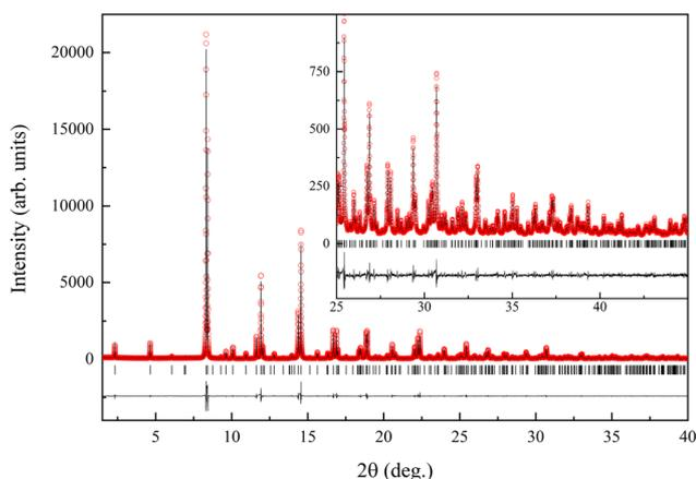
Fig. 1 Rietveld fit to synchrotron X-ray powder diffraction data ( $\lambda = 0.41376$  Å) of Eu<sub>3</sub>Ta<sub>2</sub>ON<sub>5</sub>, performed in the  $I4/mmm$  space group with  $a = 3.98240(1)$ ,  $c = 20.42020(6)$  Å. The inset shows the high  $2\theta$  region enlarged.
