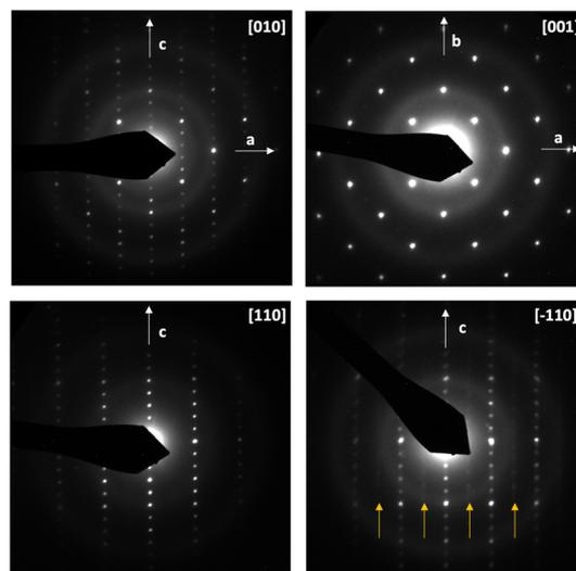
Fig. 2 Electron diffraction patterns of Eu<sub>3</sub>Ta<sub>2</sub>ON<sub>5</sub> along [010], [001] and [110] axes. Orange arrows indicate superstructure reflections observed in some crystals, that can be indexed in a  $\sqrt{2}a_0 \times \sqrt{2}a_0 \times c_0$  unit cell.
