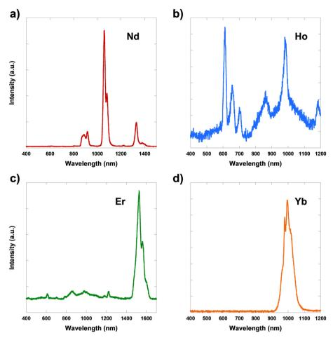
Fig. 8 Emission spectra of (a) complexes 1 ( $\lambda_{ex}$  = 380 nm), (b) 2 ( $\lambda_{ex}$  = 380 nm), (c) 3 ( $\lambda_{ex}$  = 380 nm), and (d) 4 ( $\lambda_{ex}$  = 380 nm) in MeCN solution at room temperature.
