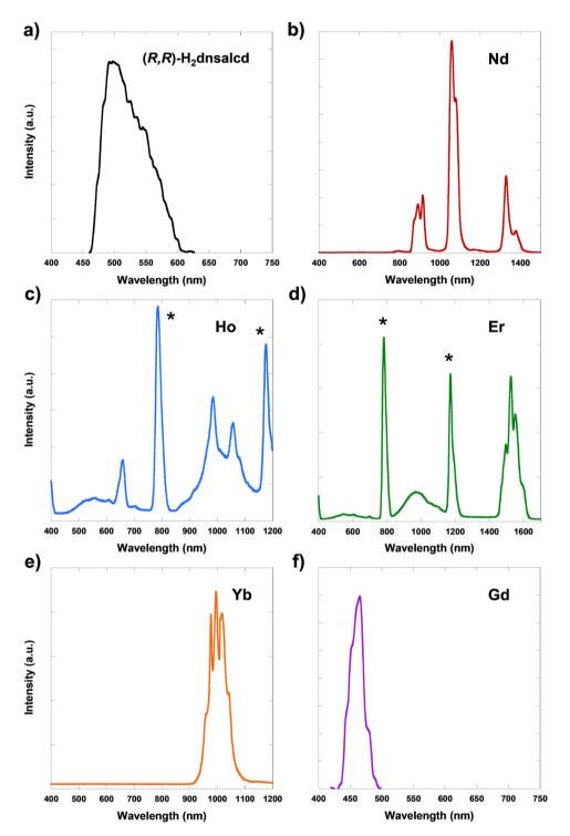
Fig. 6 Emission spectra of (a) (R,R)-H<sub>2</sub>dnsalcd  $(\lambda_{ex}$  = 390 nm) and (b) complexes 1  $(\lambda_{ex}$  = 380 nm), (c) 2  $(\lambda_{ex}$  = 380 nm), (d) 3  $(\lambda_{ex}$  = 380 nm), (e) 4  $(\lambda_{ex}$  = 380 nm), and (f) 5  $(\lambda_{ex}$  = 400 nm) in the solid state at room temperature. \* indicates Rayleigh scattering peaks.
