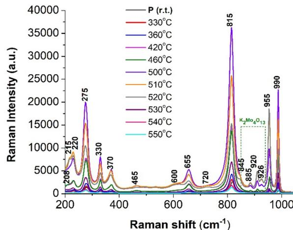
Fig. 1 *In situ* Raman spectra of pristine **P** at temperatures ranging from room temperature up to 550 °C. The green dashed lines indicate the region of bands assigned to the  $K_2Mo_4O_{13}$  crystalline phase.
