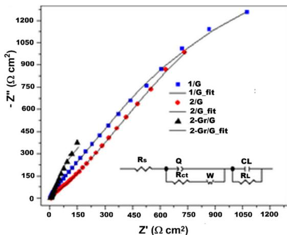
**Fig. 11** Nyquist plots of 1/G, 2/G and 2-Gr/G and their simulated curves (solid lines). The inset shows the electrical equivalent circuit used to simulate the impedance spectra. The equivalent considers the solution resistance  $R_s$ , the charge transfer characteristics  $R_{ct}$ , the constant phase element of the double layer  $Q$ , the Warburg element  $W$ , and the leakage resistance  $R_l$  associated in parallel with CL.
