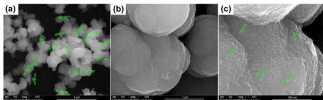
**Fig. 3** FE-SEM images for sample 1 at different magnifications: (a) overall view ( $\times 20\,000$ ) and (b and c) details ( $\times 50\,000$  and  $\times 100\,000$ , respectively); green dashed ellipses in (c) indicate conglomerates formed by the self-assembly phenomena of elongated particles.
