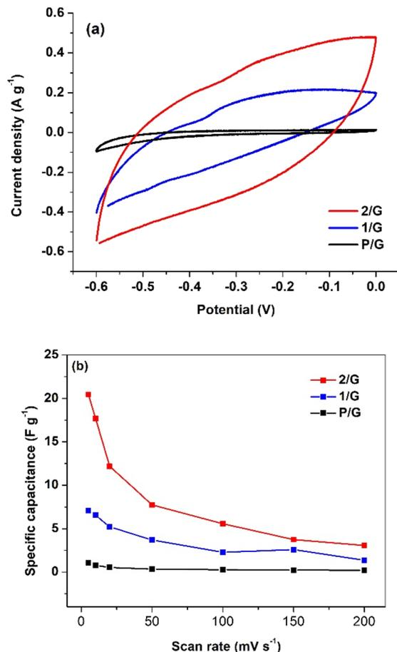
Fig. 7 (a) Overlapped CV plots for P/G, 1/G and 2/G modified electrodes recorded at a  $20 \text{ mV s}^{-1}$  sweep rate. (b) The variation of gravimetric capacitance values,  $C$ , of P/G, 1/G and 2/G modified electrodes with the sweep rate,  $v$ , using  $0.5 \text{ M}$  aqueous solution of  $\text{Na}_2\text{SO}_4$  as the electrolyte (the lines are guides for the eye).
