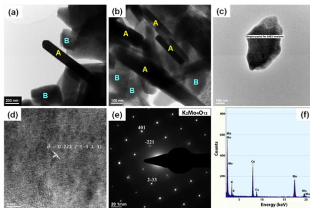
**Fig. 5** (a and b) Bright-field global TEM images of different magnifications for 1 (400 °C): (A)  $\alpha$ -MoO<sub>3</sub> and (B) K<sub>2</sub>Mo<sub>4</sub>O<sub>13</sub> crystals, (c) bright-field detailed TEM image of a K<sub>2</sub>Mo<sub>4</sub>O<sub>13</sub> single crystal, and (d) HR-TEM image, (e) SAED pattern and (f) EDX spectrum recorded on the single crystal depicted in (c).
