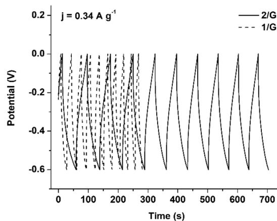
Fig. 8 GCD curves of 2/G and 1/G at an applied current density of  $0.34 \text{ A g}^{-1}$  in  $0.5 \text{ M}$   $\text{Na}_2\text{SO}_4$ .
