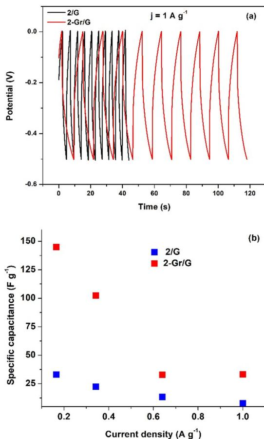
Fig. 10 (a) Overlapped GCD curves of 2-G and 2-Gr/G at an applied current density of 1 A g<sup>-1</sup> in 0.5 M aqueous solution of Na<sub>2</sub>SO<sub>4</sub> ( $j$  is the current density). (b) Gravimetric capacitances at various current densities for 2-G and 2-Gr/G in 0.5 M aqueous solution of Na<sub>2</sub>SO<sub>4</sub>.
