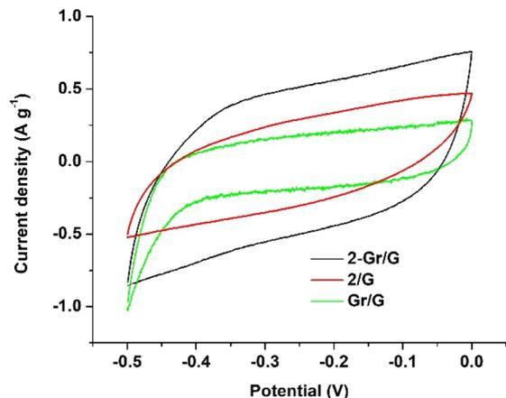
Fig. 9 CVs of 2-Gr/G, 2/G and Gr/G at 20 mV s<sup>-1</sup> in 0.5 M aqueous solution of Na<sub>2</sub>SO<sub>4</sub>.
