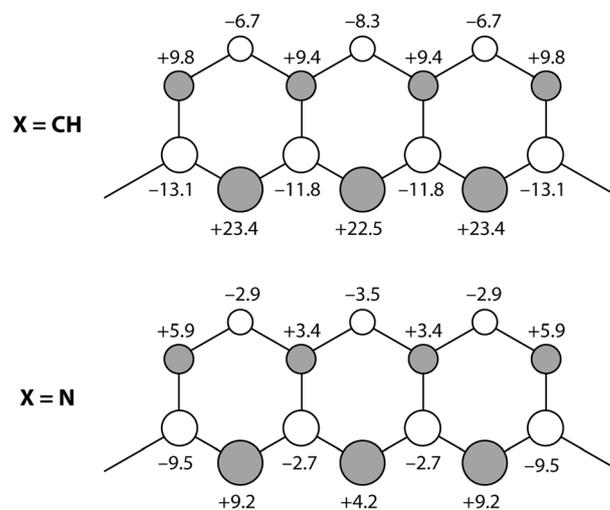
**Fig. 9** Schematic representation of the local spin density distribution on the bridging pathways for  $N = 3$  ideal models with oligoacene and pyridine-oligoacene spacers. Full and empty contours denote positive and negative values of the spin density. Calculated atomic densities in  $me^-$  are given in parentheses.
