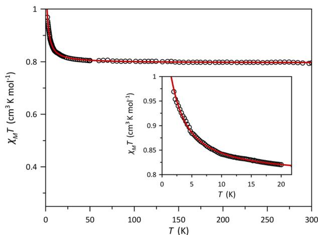
Fig. 5 Thermal dependence of  $\chi_{\text{M}}T$  for **1**: (empty circles) experimental; (solid line) best-fit curve through the Bleaney–Bowers equation. The inset shows details of the low-temperature region.
