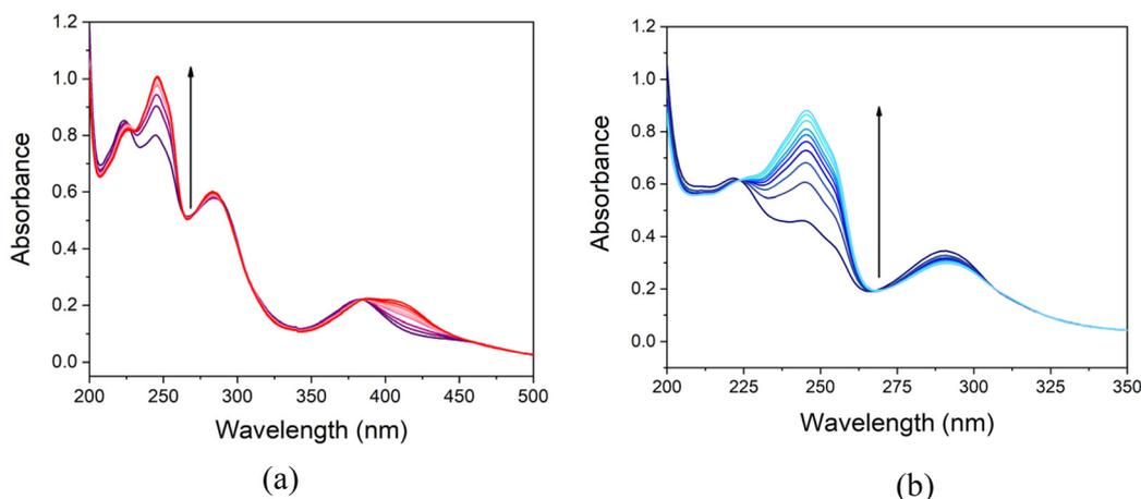
Fig. 3 Evolution of the electronic absorption spectra of the oxidation of H<sub>2</sub>Q into BQ ( $\lambda_{\max} = 245$  nm) catalysed by **1** (a) and **3** (b) at 25 °C under dioxygen saturation. The arrows indicate the course of the reaction during one hour.  $[\text{H}_2\text{Q}]_0 = 75 \mu\text{mol L}^{-1}$  and  $[\mathbf{1}] = [\mathbf{3}] = 7.5 \mu\text{mol L}^{-1}$ .
