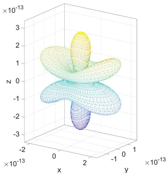
**Fig. 6** Three-dimensional projection of the representation surfaces of tensor  $d'_{333} = \alpha_{3i}\alpha_{3j}\alpha_{3k}d_{ijk}$  for  $[\text{ScCl}_2(18\text{c}6)][\text{AlCl}_4]$  (**4**) (for two-dimensional projections of the representation surfaces see ESI: Fig. S8†). The  $\alpha_{3i}$ ,  $\alpha_{3j}$  and  $\alpha_{3k}$  are direction cosines.
