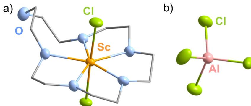
Fig. 5 Crystal structure of  $[\text{ScCl}_2(18\text{c}6)][\text{AlCl}_4]$  (4): (a)  $[\text{ScCl}_2(18\text{c}6)]^+$  cation, (b)  $[\text{AlCl}_4]^-$  anion (hydrogen atoms and disorder not shown for clarity).
