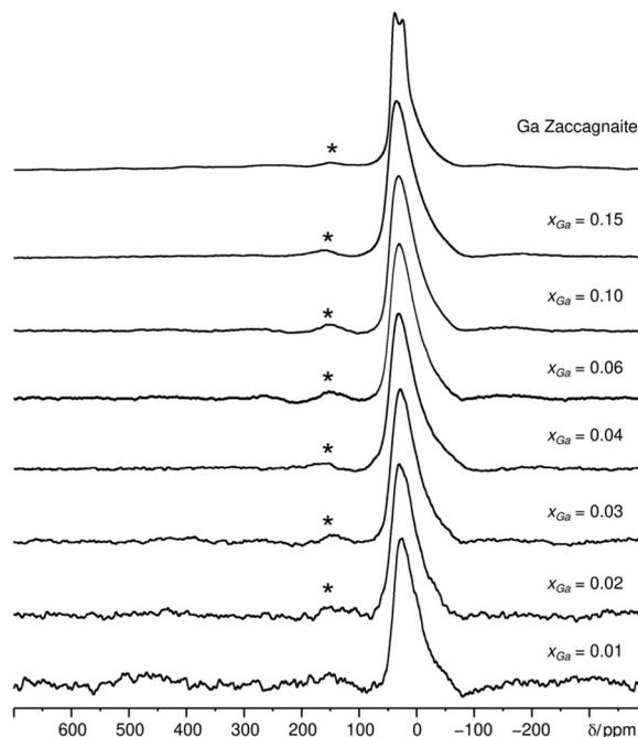
Fig. 3 Scaled  $^1\text{H}$  decoupled  $^{71}\text{Ga}$  MAS NMR stackplot of gallium doped hydrozincite and a zaccagnaite-like Zn,Ga LDH phase ("Ga Zaccagnaite"). The gallium content for the hydrozincites is given by  $x_{\text{Ga}}$ . All spectra were recorded with a spinning frequency of 20 kHz.
