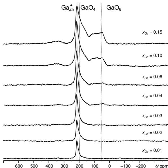
Fig. 7  $^1\text{H}$  decoupled  $^{71}\text{Ga}$  MAS NMR stackplot of doped zinc oxide, annealed at 320 °C for 4 h, with different cation-based molar gallium fractions,  $x_{\text{Ga}}$ . All spectra were recorded with a spinning frequency of 20 kHz.
