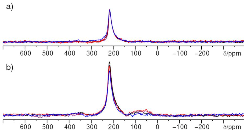
**Fig. 12**  $^1\text{H}$  decoupled  $^{71}\text{Ga}$  PASPA MAS NMR of ZnO:Ga with  $x_{\text{Ga}} = 0.03$  (a) and  $x_{\text{Ga}} = 0.1$  (b) recorded at 20 kHz rotation frequency, comparing the as-made sample (purple spectrum) to the reference sample (black spectrum), the acetonitrile blind test sample (red spectrum) and the paramagnetically impregnated sample (blue spectrum).
