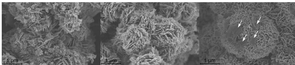
Fig. 6 SEM micrographs of selected ZnO:Ga samples with  $x_{\text{Ga}} = 0.01$  (left), 0.04 (center) and 0.15 (right). Larger platelets observed in the sample with  $x_{\text{Ga}} = 0.15$  are marked with arrows.
