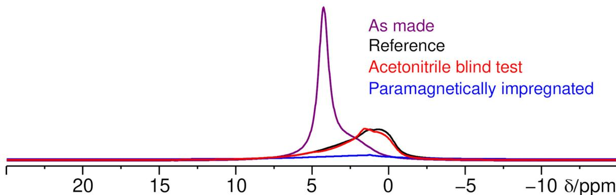
**Fig. 13**  $^1\text{H}$  PASPA MAS NMR of ZnO:Ga with  $x_{\text{Ga}} = 0.03$  recorded at 20 kHz rotation frequency, comparing the as-made sample (purple) to the reference sample (black), the acetonitrile blind test sample (red) and the paramagnetically impregnated sample (blue).
