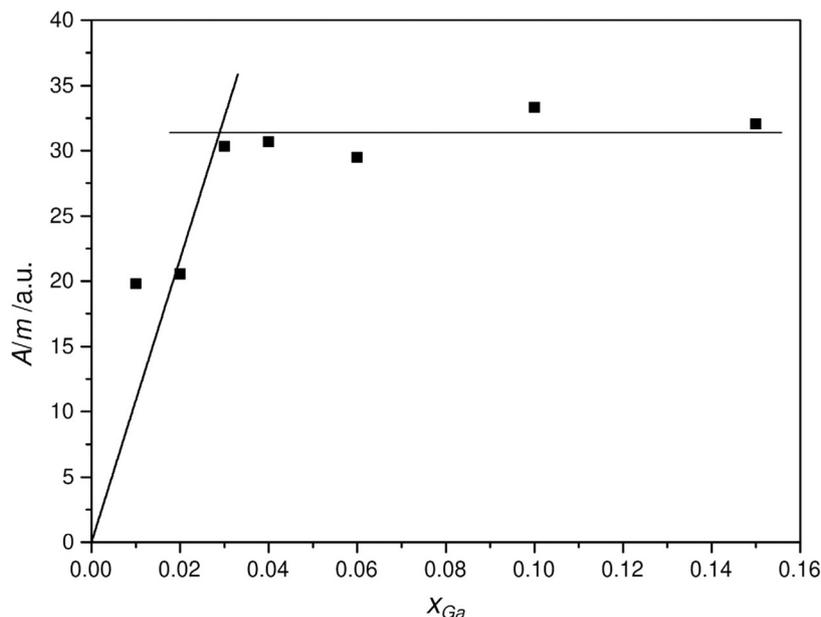
**Fig. 11** Ratio of the  $^{71}\text{Ga}$  MAS NMR signal area per mass  $A/m$  for the signal at  $\delta_{\text{iso}}^{\text{exp}} = 213$  ppm of ZnO:Ga, annealed with 320 °C for 4 h with different cation-based molar gallium fractions  $x_{\text{Ga}}$ . The NMR spectra were excited with a selective  $\pi/2$  pulse. The lines to interpolate the substitution limit were obtained by fitting linear functions into the corresponding data points.
