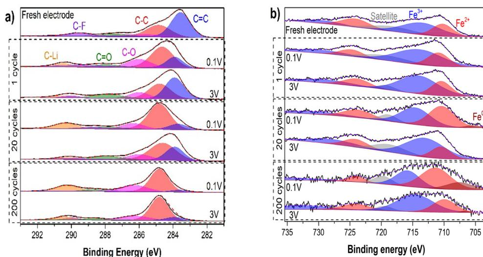
Fig. 3 XPS high-resolution (a) C 1s and (b) Fe 2p spectra of a fresh electrode and of lithiated/delithiated electrodes stopped at the galvanostatic cycles 1<sup>st</sup>, 20<sup>th</sup> and 200<sup>th</sup>.
