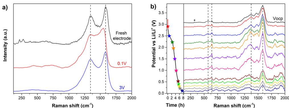
**Fig. 5** (a) *Ex situ* Raman measurements of two fully activated electrodes stopped at 0.1 V (lithiated) and 3 V (delithiated) and a fresh non-cycled electrode. The three spectra have been normalized to facilitate comparison. (b) *Operando* Raman spectra of the first galvanostatic lithiation measured at the voltages indicated in the plot profile on the left. The asterisk indicates the peak from the CaF<sub>2</sub> window of the Raman cell used for the *operando* Raman measurements.
