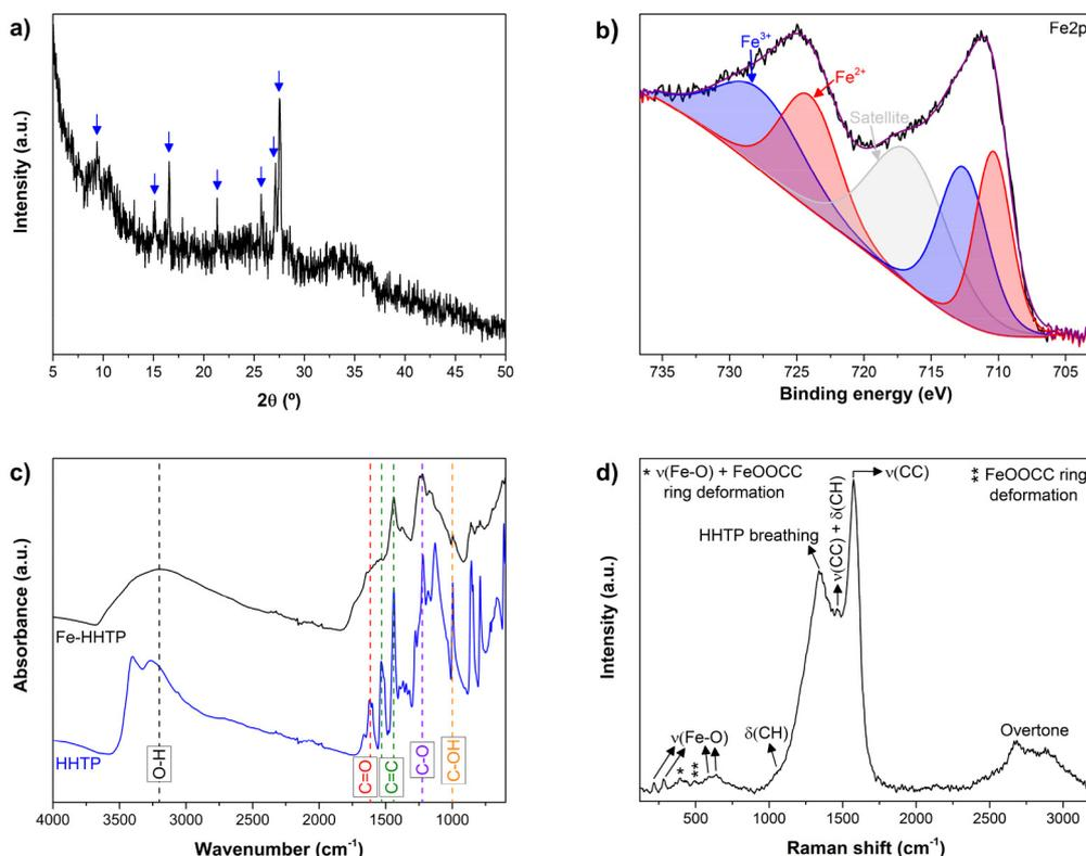
**Fig. 1** Characterization of the synthesized Fe-HHTP powders including (a) PXRD pattern with blue lines indicating the peak positions, (b) XPS high-resolution Fe 2p graph, (c) comparison between Fe-HHTP and HHTP infrared spectrum and (d) Raman spectrum.
