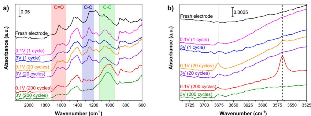
Fig. 4 Infrared spectra of fresh and cycled electrodes stopped at 0.1 V (lithiated) and 3 V (delithiated) showing the regions (a) from 2170 cm<sup>-1</sup> to 600 cm<sup>-1</sup> and (b) from 3740 cm<sup>-1</sup> to 3525 cm<sup>-1</sup>.
