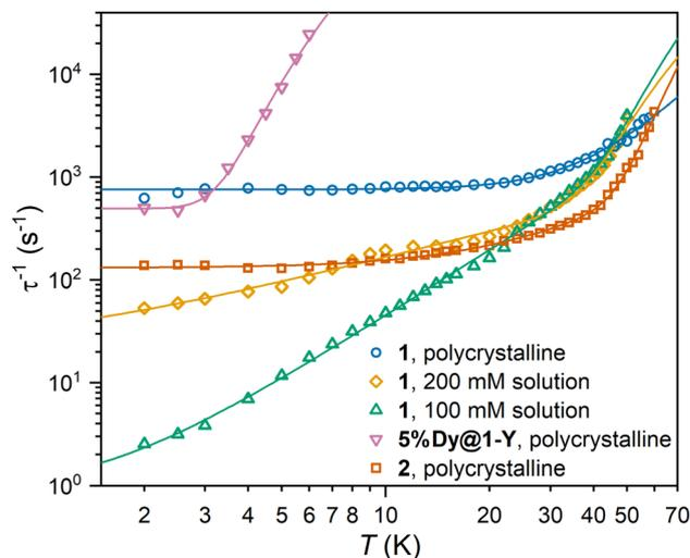
Fig. 4 Temperature-dependence of relaxation rates for **1** (blue), **2** (red), **5%Dy@1-Y** (pink) and 9 : 1 toluene/hexane frozen solutions of **1** at 200 mM (gold) and 100 mM (green). Solid lines show fit of relaxation profiles without weighting by rate distributions using the parameters in Table 2.
