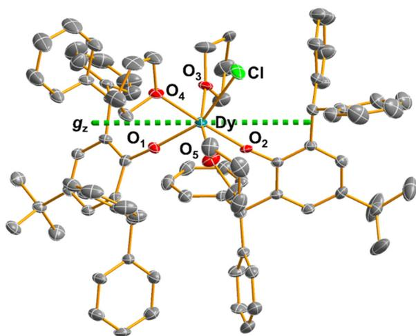
**Fig. 1** Molecular structure of **1** from single crystal XRD at 150 K with thermal ellipsoids drawn at 40% probability level and selective atom labelling (Dy teal, Cl green, O red, C grey). Dotted green line represents the calculated principal magnetic axis for **1**. H atoms and lattice solvent are omitted for clarity.
