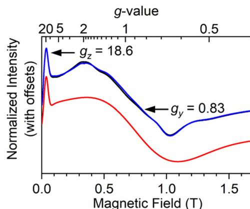
**Fig. 2** Continuous wave X-band ( $\nu = 9.379332$  and  $9.380314$  GHz) EPR powder spectra of **1** at 6.9 K showing two experimental spectra at approximately perpendicular sample rotations (black, blue) and simulation (red).
