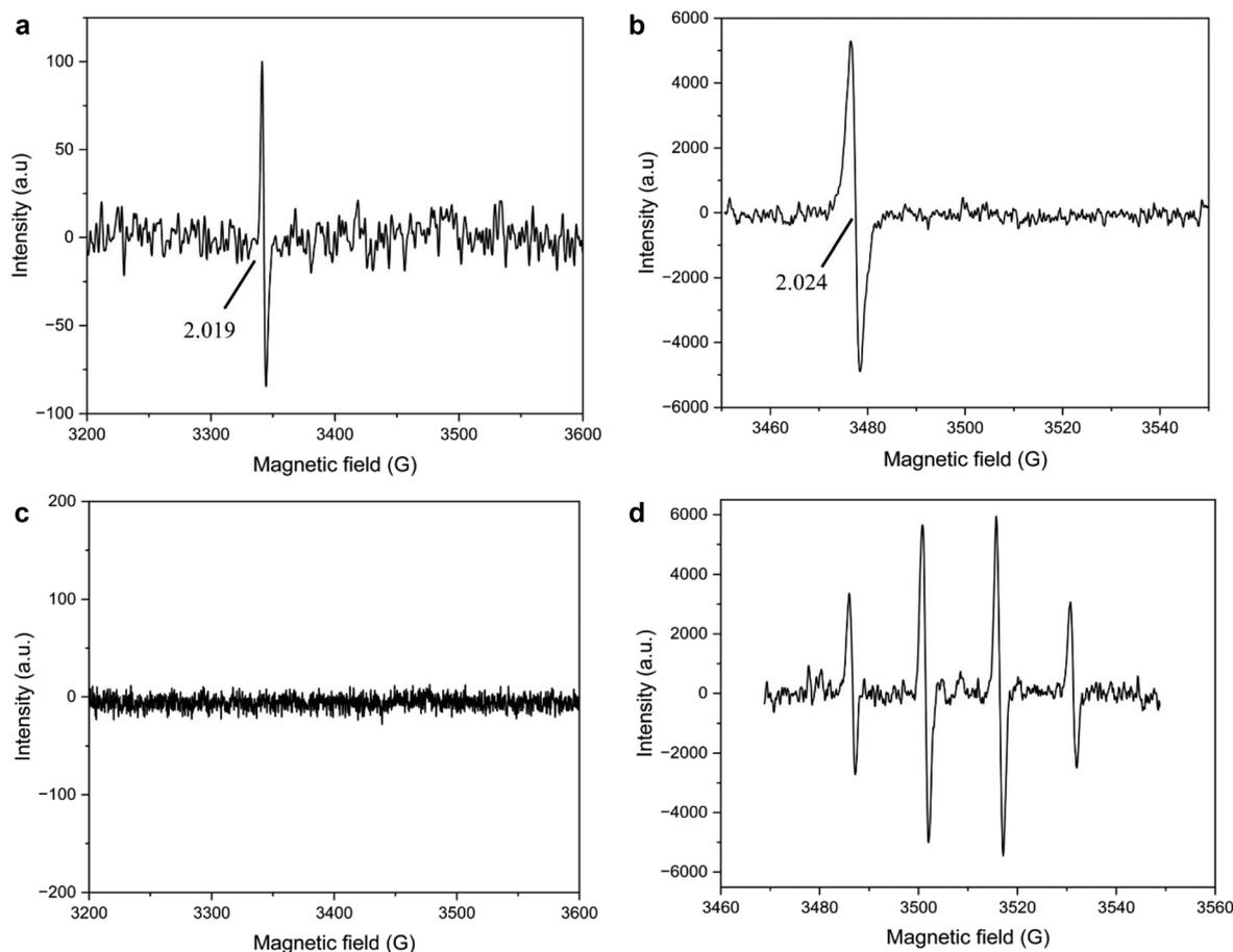
**Fig. 5** EPR spectra are reported for (a) solid  $\text{NaU}_{24}$ , (b)  $\text{NaU}_{24}$  dissolved in water, (c)  $\text{NaU}_{24}$  dissolved in water and spectra collected after 30 minutes of aging, and (d)  $\text{NaU}_{24}$  dissolved in water with the DMPO spin trap agent.
