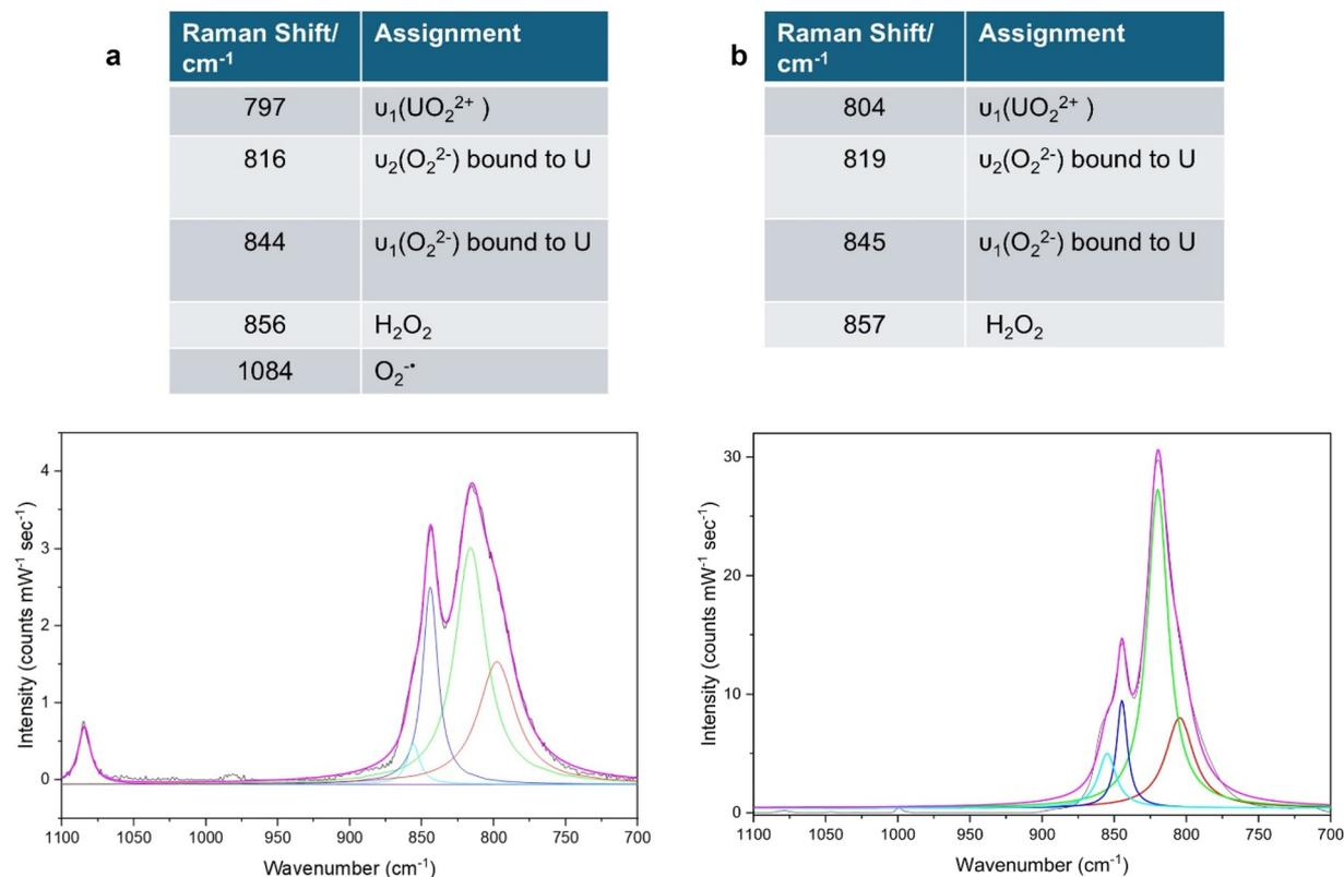
Fig. 4 (a) Raman spectra of the solid NaU<sub>24</sub> cluster as synthesized and (b) after being washed with hexane show a decrease in the band at 1084 cm<sup>-1</sup> and a relative increase in the band at 857 and 819 cm<sup>-1</sup>.
