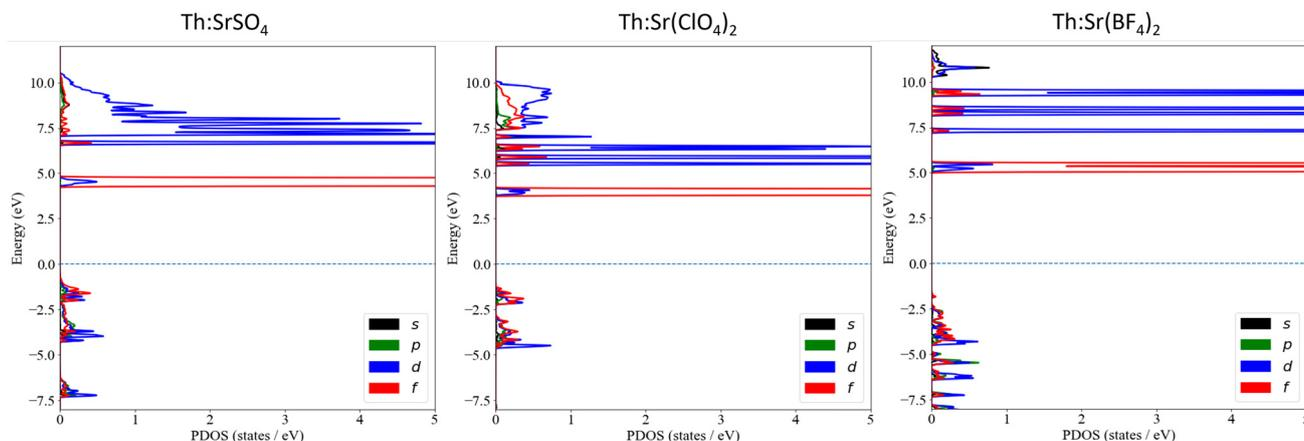
Fig. 3 Thorium projected density of states plots for  $\text{Th}:\text{SrSO}_4$ ,  $\text{Th}:\text{Sr}(\text{ClO}_4)_2$ , and  $\text{Th}:\text{Sr}(\text{BF}_4)_2$ .
