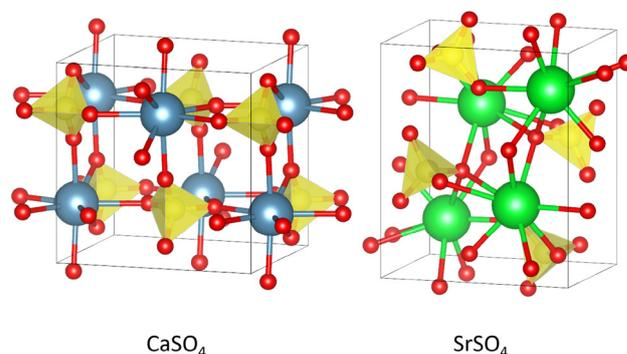
Fig. 1 Unit cells of sulfates  $\text{CaSO}_4$  and  $\text{SrSO}_4$ .
