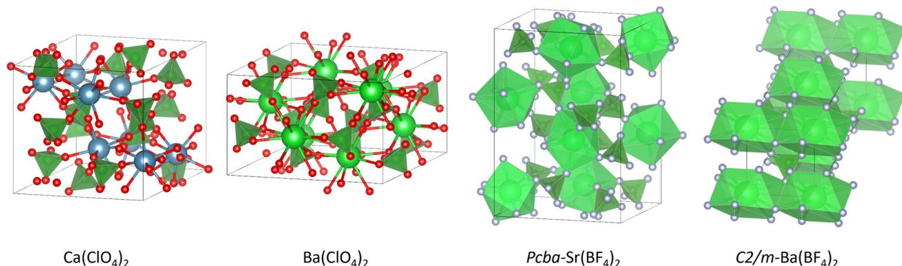
**Fig. 2** Optimized unit cells of Ca(ClO<sub>4</sub>)<sub>2</sub>, Ba(ClO<sub>4</sub>)<sub>2</sub>, *Pcba*-Sr(BF<sub>4</sub>)<sub>2</sub> (high square antiprismatic SrF<sub>8</sub>), and *C2/m*-Ba(BF<sub>4</sub>)<sub>2</sub> (showing pentagonal antiprismatic BaF<sub>10</sub>).
