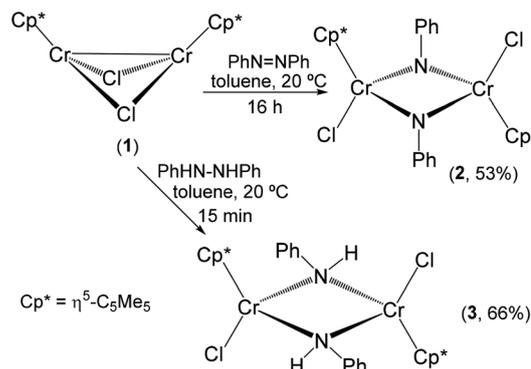
Scheme 1 Reactions of **1** with azobenzene and 1,2-diphenylhydrazine.
