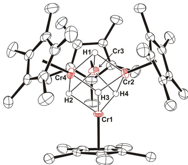
**Fig. 2** Perspective view of **4** with thermal ellipsoids at the 50% probability level. Hydrogen atoms of the  $\eta^5$ -C<sub>5</sub>Me<sub>5</sub> ligands are omitted for clarity. Selected lengths (Å) and angles (°): Cr...Cr 2.509(1)–2.753(1), Cr–H 1.72(6)–2.07(5), Cr–Cm av. 1.920(3), Cr–Cr–Cr 55.9(1)–65.3(1), H–Cr–H 79(2)–96(3), Cr–H–Cr 82(2)–103(3).
